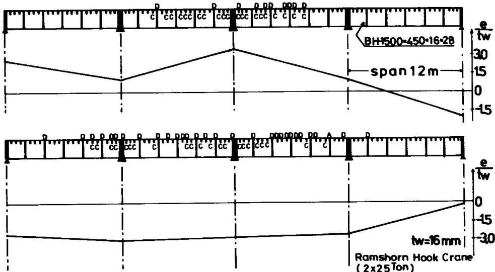
Fig.1 An example of the relation between the location of fatigue crack initiated and the eccentricity of crane rail
