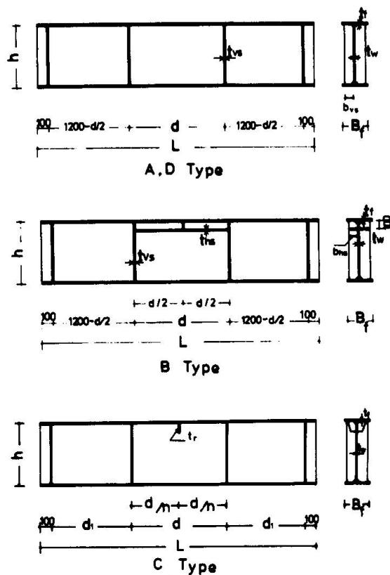
Fig.3 Tested specimens
