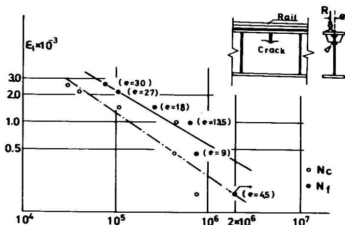
Fig.6 Fatigue test results of the Type C crack
