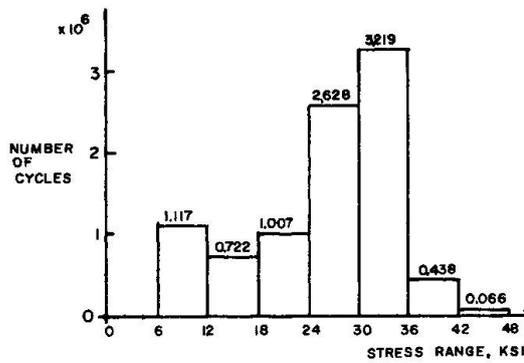
Fig. 5 Histogram of Stress Ranges; Location M7U, Gage 14
