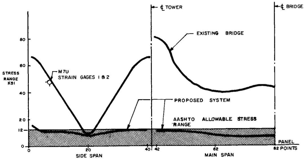
Fig. 7 Stress Ranges at Upper Roadway Floor Beams
