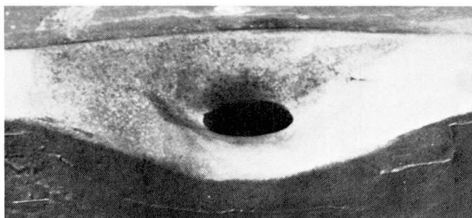
All cracks in the longitudinal weldments were removed by either grinding, drilling or coring. Figure 10 shows a retrofitted region after removal of a crack. The ground area was checked by liquid penetrant to ensure that no crack tip remained in the structure.
