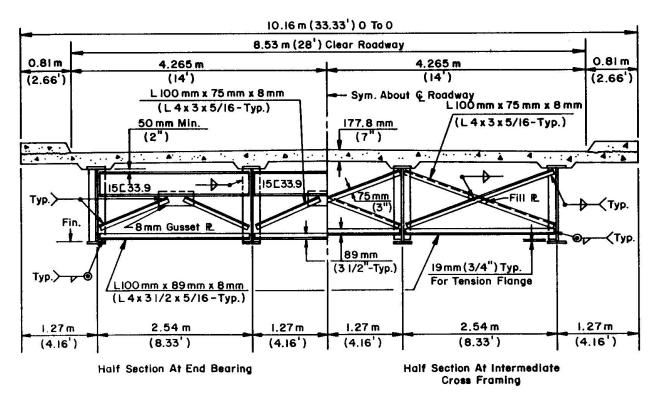
Fig. 3 The Cross-Section of the Bridge
