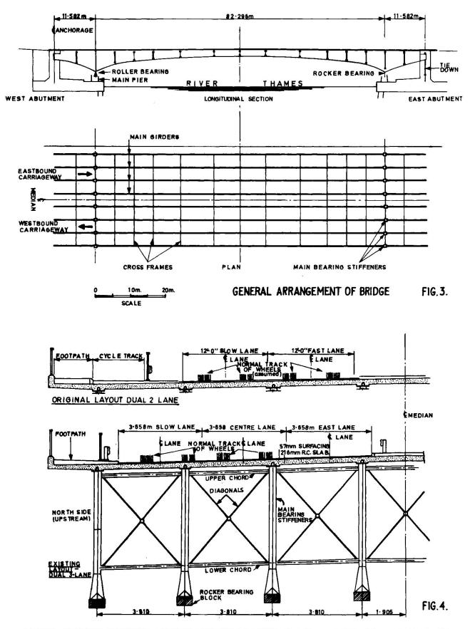
CROSS-SECTION THROUGH SUPERSTRUCTURE AT PIER UNDER EASTBOUND CARRIAGEWAY
