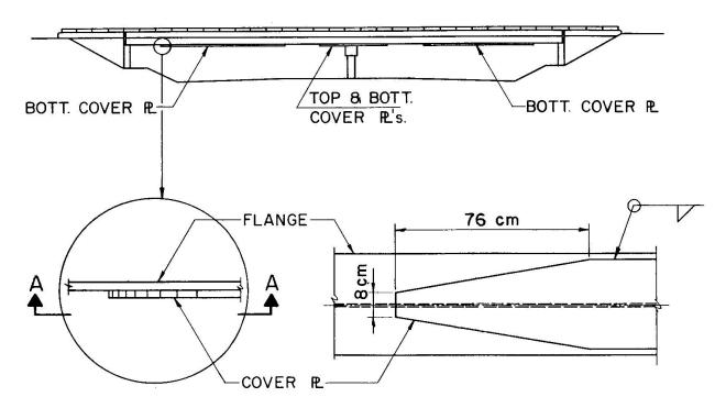
Figure 2 -- Typical End Detail of Welded Cover Plate
