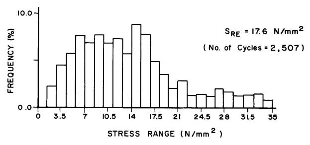
Figure 3 -- Histogram of Stress Range Spectrum for Gage No. 6
