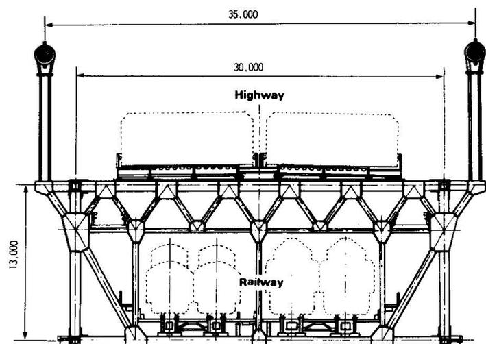
Fig1. Cross-Section of suspension bridge (Kojima-Sakaide Route)
