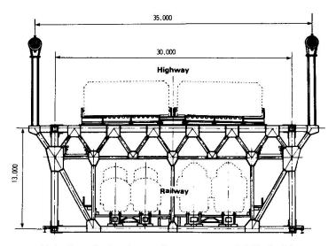
Fig.1. Cross-Section of suspension bridge (Kojima-Sakaide Route)
