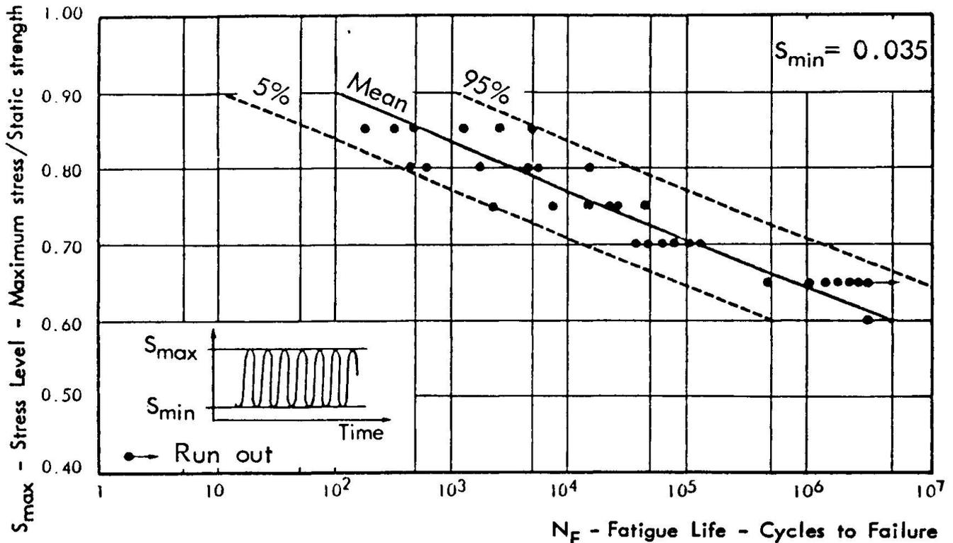
Fig. 3 Typical S-N relationship for concrete in compression
