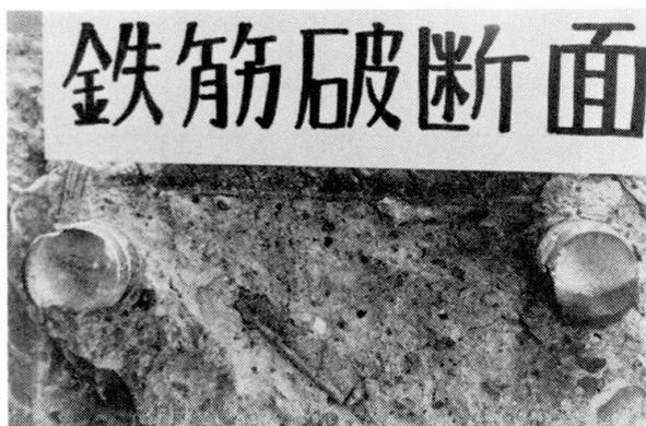
Photo. 2 Fracture Surface of Bar
