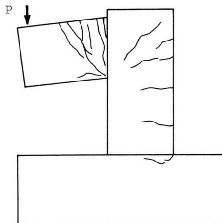
Fig. 4 Crack Pattern (at  $\delta = 4\delta_y$ )
