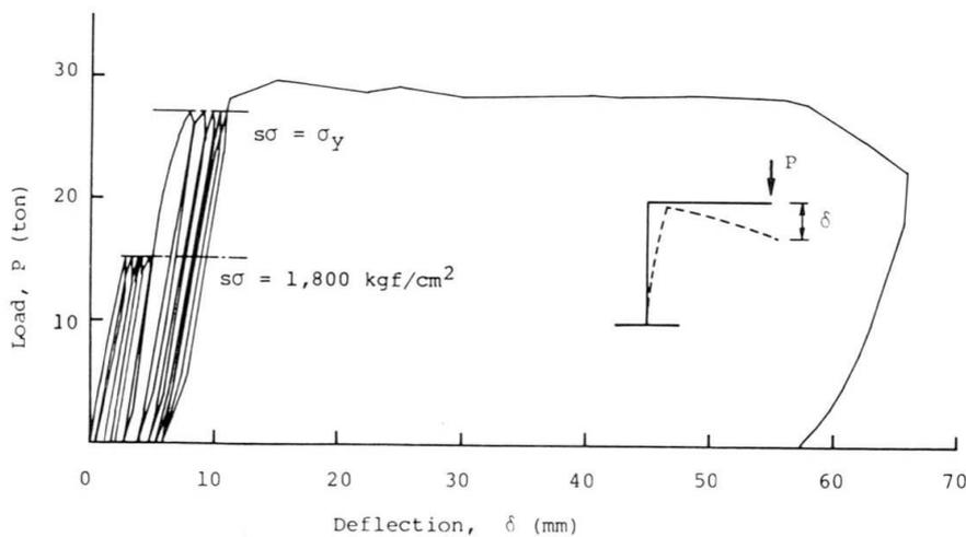
Fig. 2 Load-Deflection Curve (Static Test)
