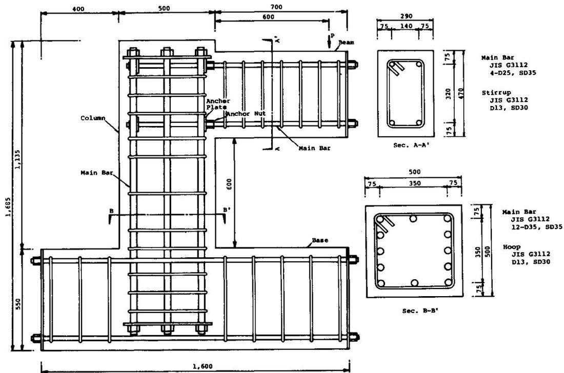
Fig. 1 Details of Specimens (in mm)
