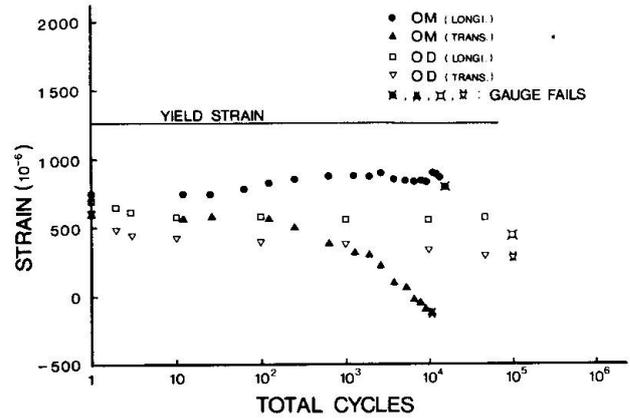
Fig. 7 Strain Variations under Load 29 kN.
