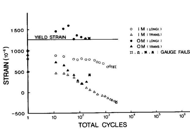
Fig. 6 Strain Variations under Load 39 kN.
