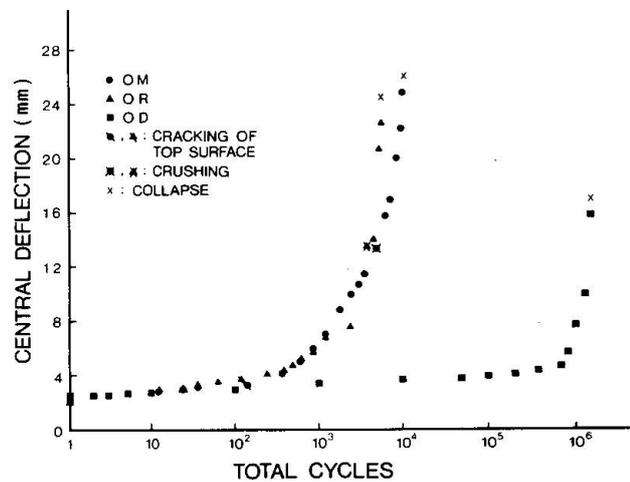
Fig. 5 Growth of Central Deflection under Load 34.3 kN.
