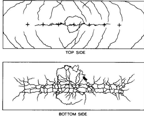
Fig. 2 Final Cracking Pattern in the Slab IM.
