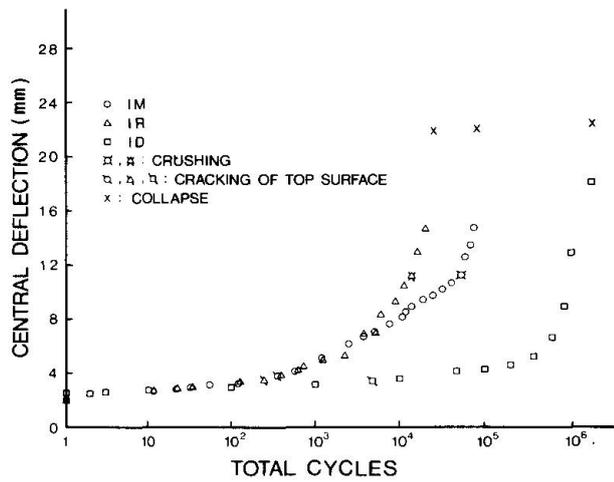
Fig. 4 Growth of Central Deflection under Load 34.3 kN.
