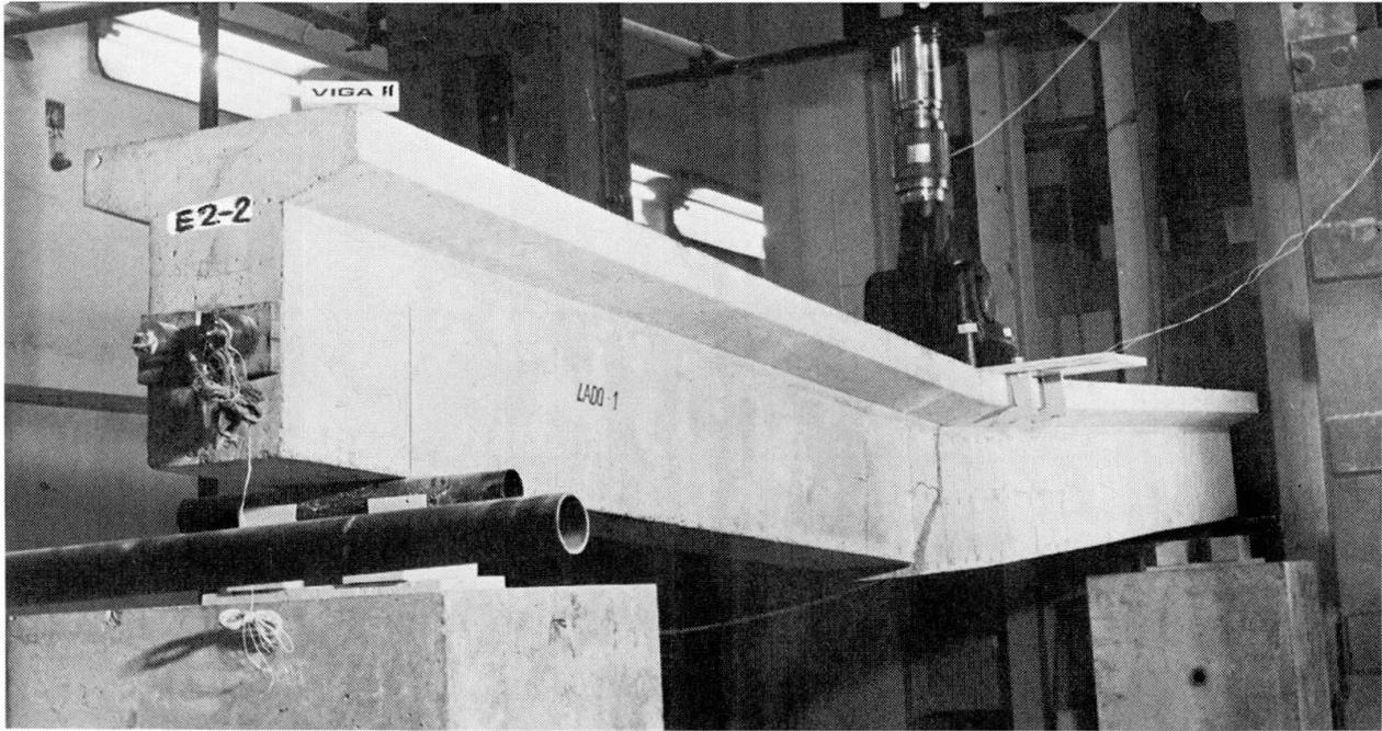
Fig. 8 Photograph of E2-2 Beam After Failure
