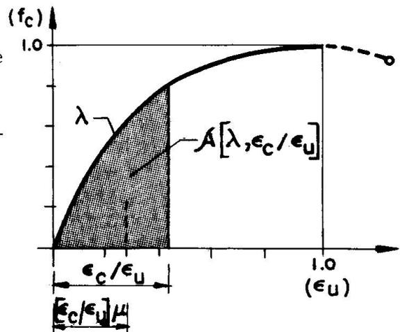
Fig. 2 Concrete Stress-Strain Curve
