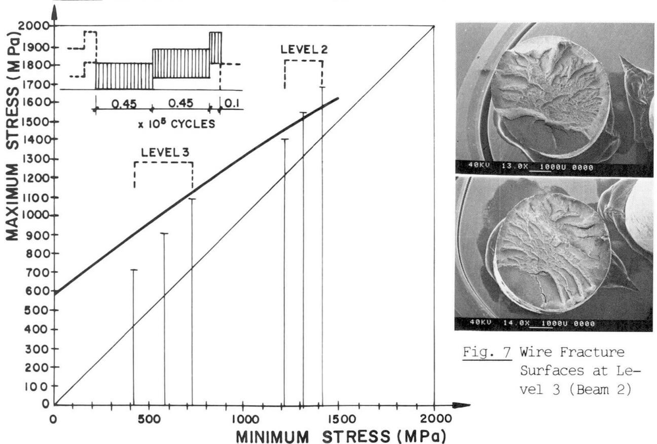
Fig. 7 Wire Fracture Surfaces at Level 3 (Beam 2)
