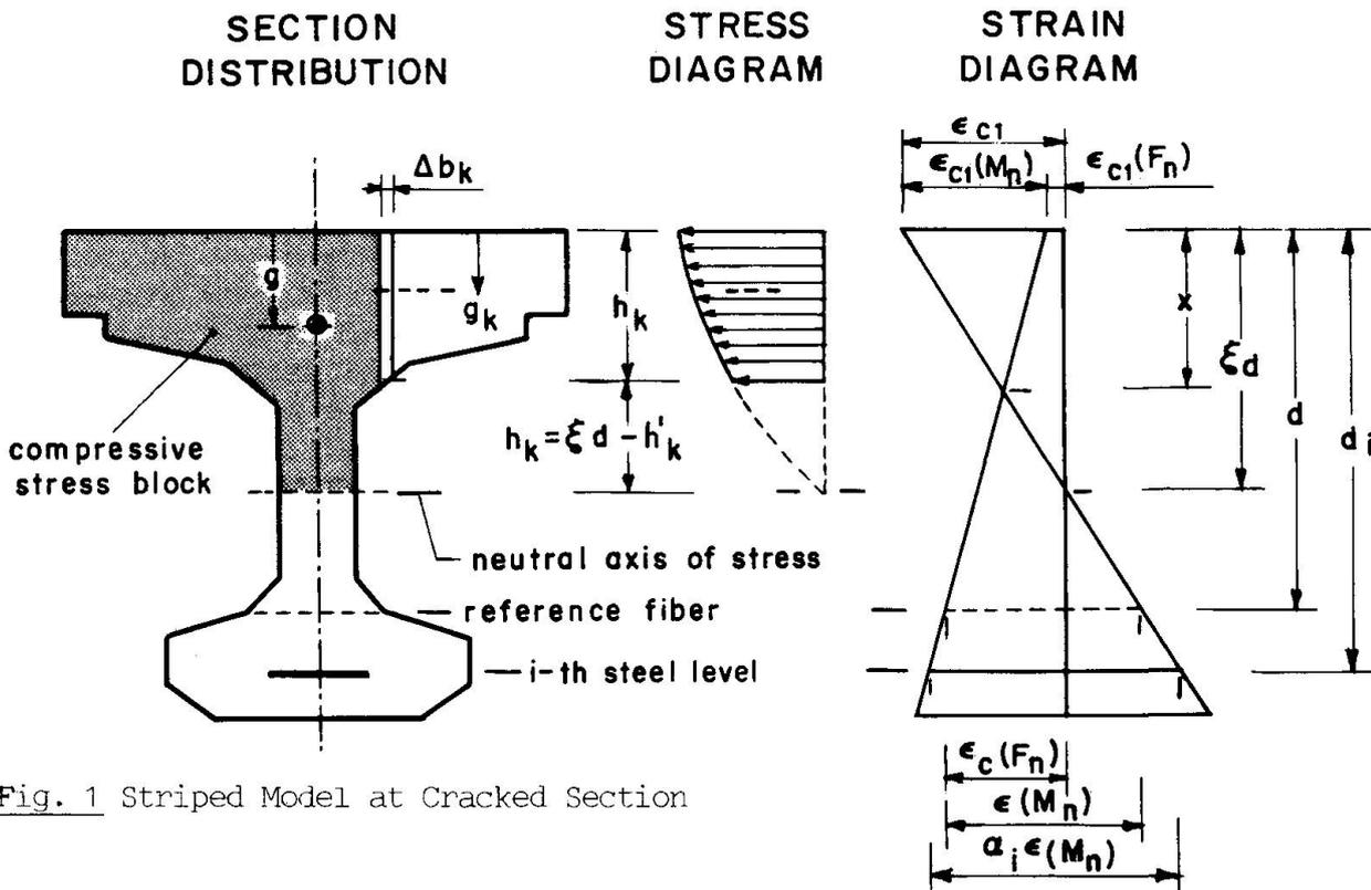
Fig. 1 Striped Model at Cracked Section
