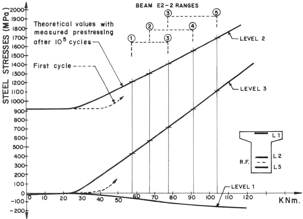
Fig. 5 Reinforcement Stresses vs. Applied Bending Moment
