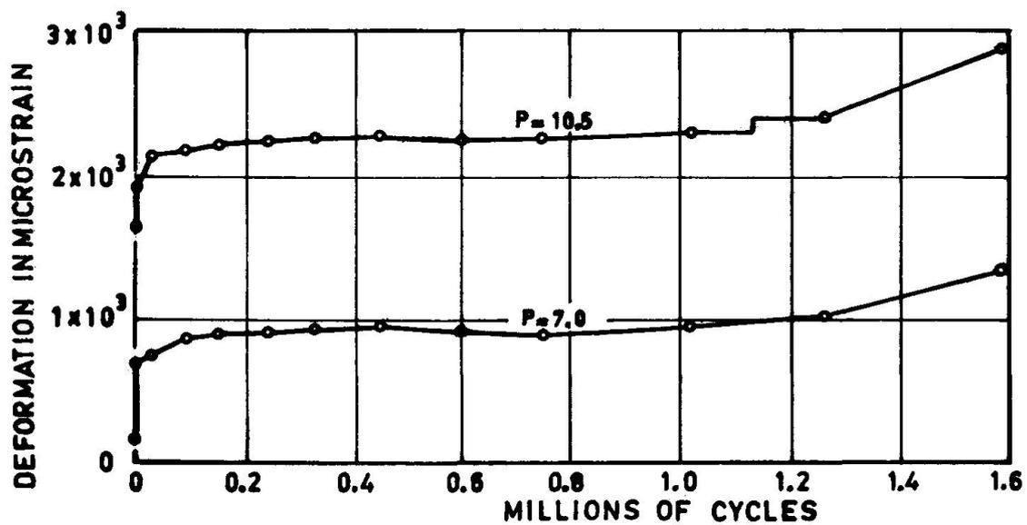
Fig 3. Concrete deformation, Beam F8 (ref. 4)
