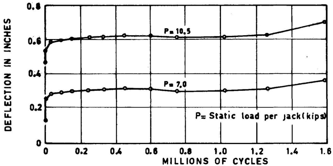
Fig 2. Mid-span deflection, Beam F8 (ref. 4)
