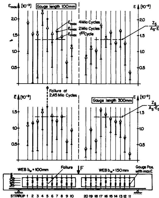
**Fig. 7:** Beam BI/3: Variation of Stirrup Strains under max. Load  $F = 370 \text{ kN}$
