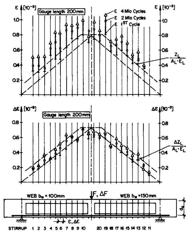
**Fig. 6:** Beam BI/3: Variation of Strains in Longitudinal Reinforcement under max. Load  $F = 370 \text{ kN}$  and under Load Range  $\Delta F = 340 \text{ kN}$
