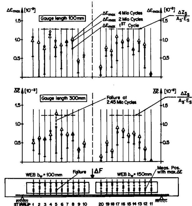
**Fig. 8:** Beam BI/3: Variation of Stirrup Strains under Load Range  $\Delta F = 340 \text{ kN}$
