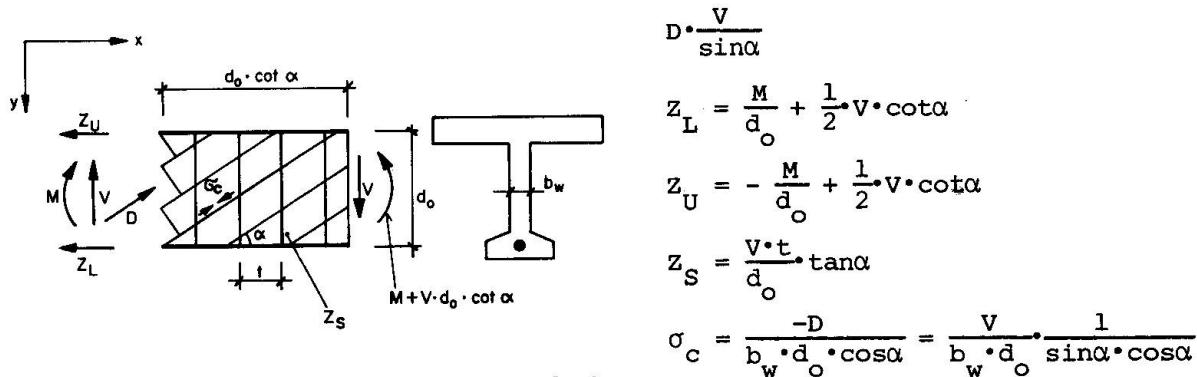
Fig. 9: Truss Model for Bending and Shear
