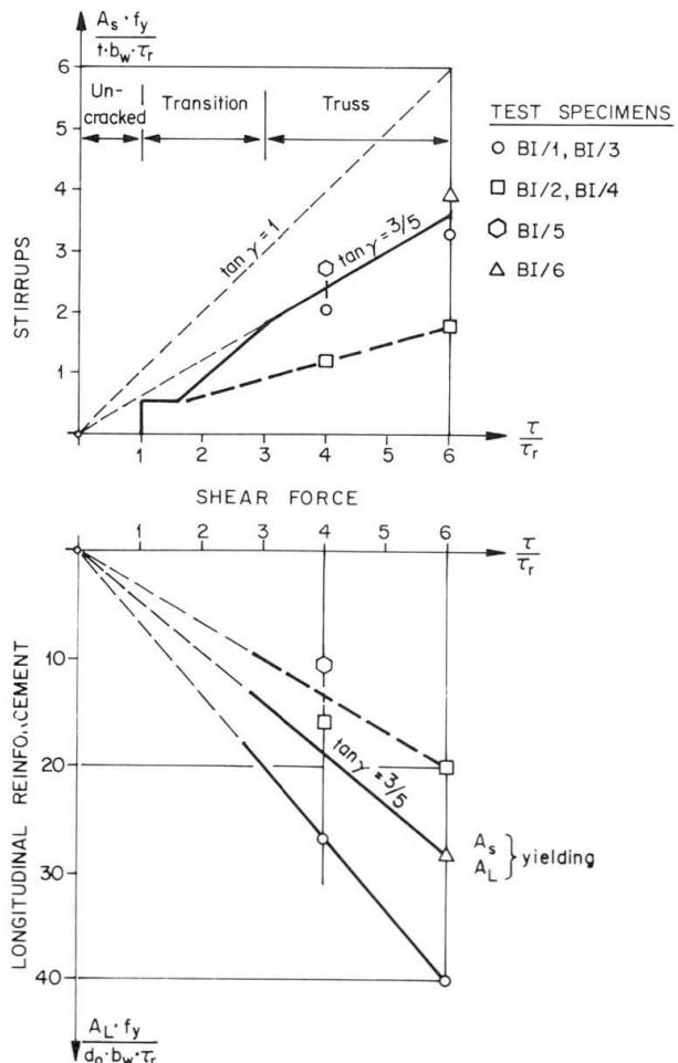
Fig. 1: Design Parameters
