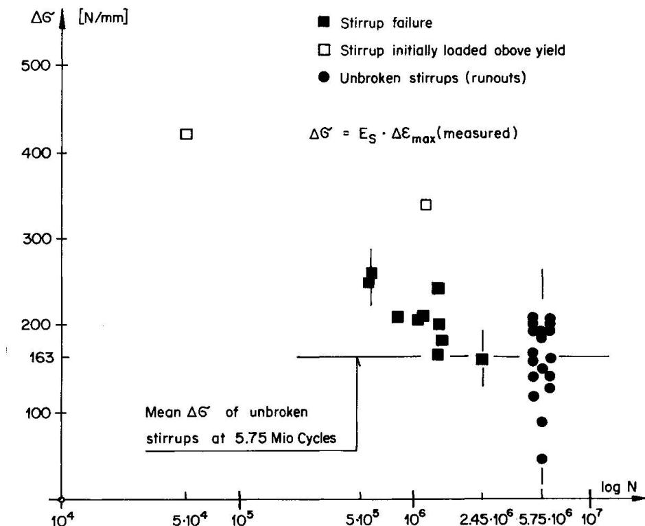
Fig. 10:  $\Delta\sigma$ -N Diagram for Stirrups, diameter 10 mm
