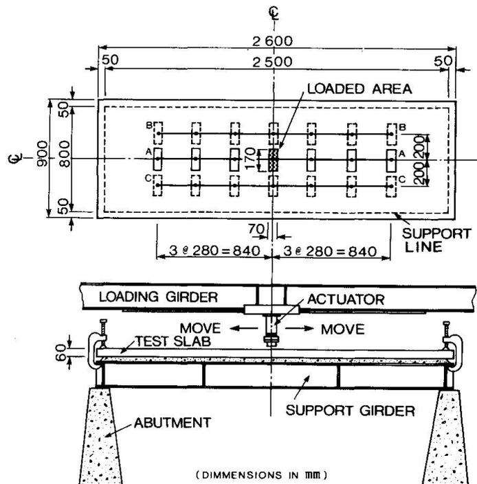
Fig. 1 Test Setup.
