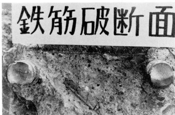
Photo. 2 Fracture Surface of Bar
