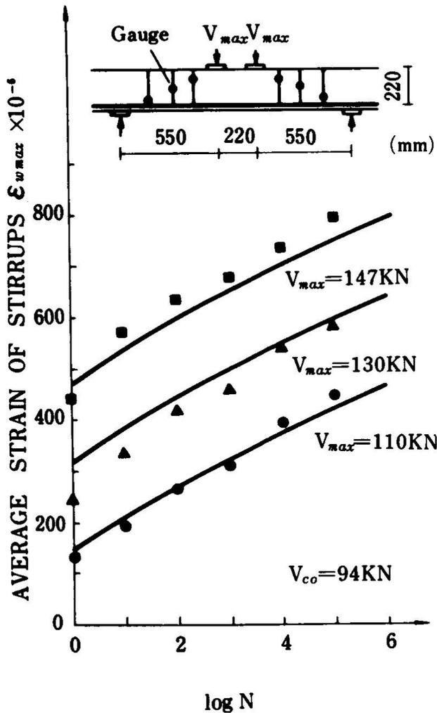
Fig.2 Average Strain of Stirrups ( $V_{max} > V_{co}$ )
