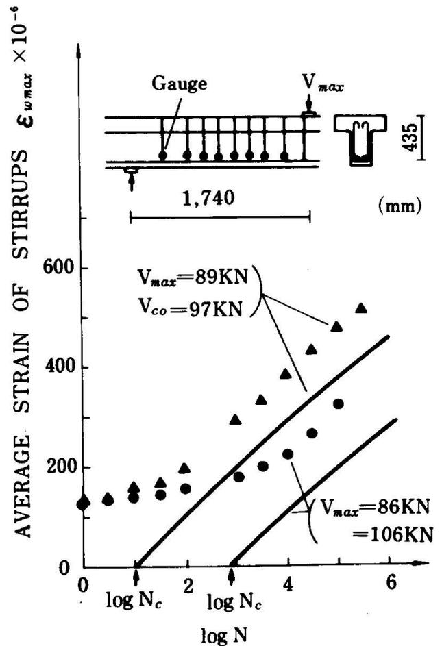
Fig.3 Average Strain of Stirrups ( $V_{max} < V_{co}$ )
