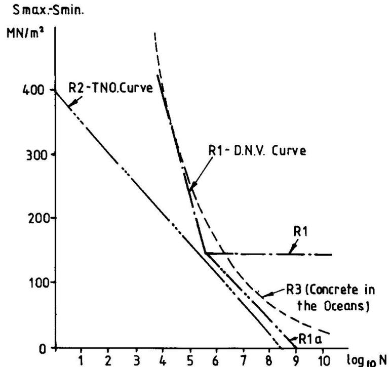
FIG.3 S-N CURVES FOR STEEL REINFORCEMENT
