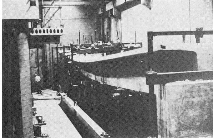
Fig. 4 - Repetitive Loading Setup Fig. 5 - Girder No. 2 at Ultimate Load.
