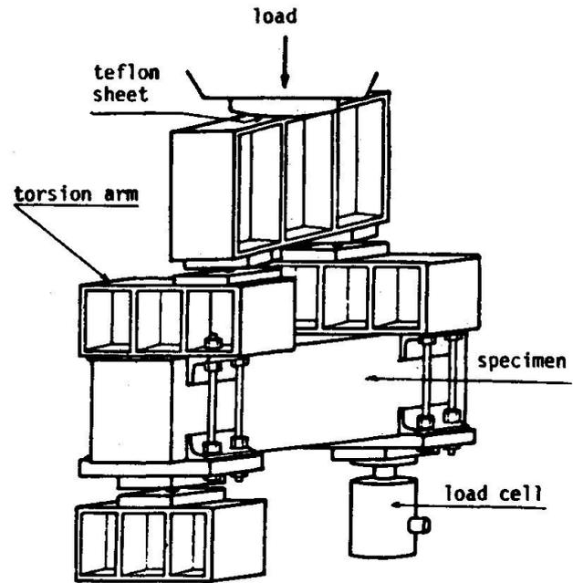
Fig.2 test arrangement
