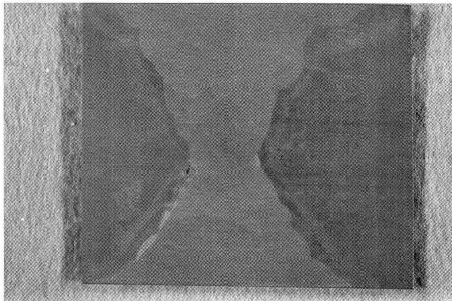
Fig. 6 Cross Section of Weld at Embedded Defect
