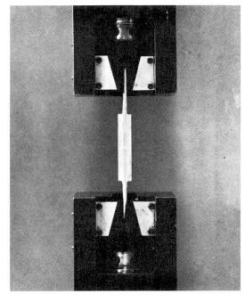
Figure 3 Lap joint under test
