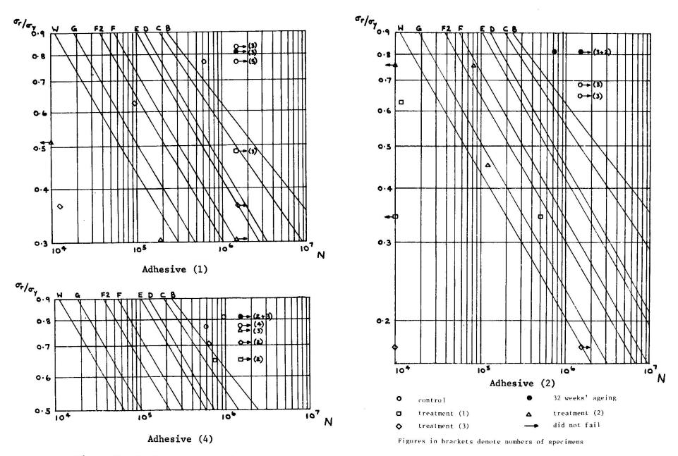
Figure 2 Fatigue test results for open sandwich beams
