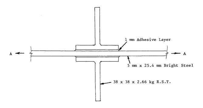
Fig 4. Test Specimen. Adhesive Bonded Unstressed T
