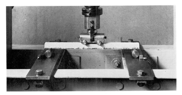
Figure 1 Open sandwich beam under test
