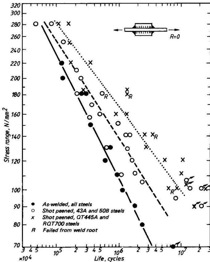
Fig. 3. Fatigue test results for shot peened specimens with longitudinal fillet welded attachments.
