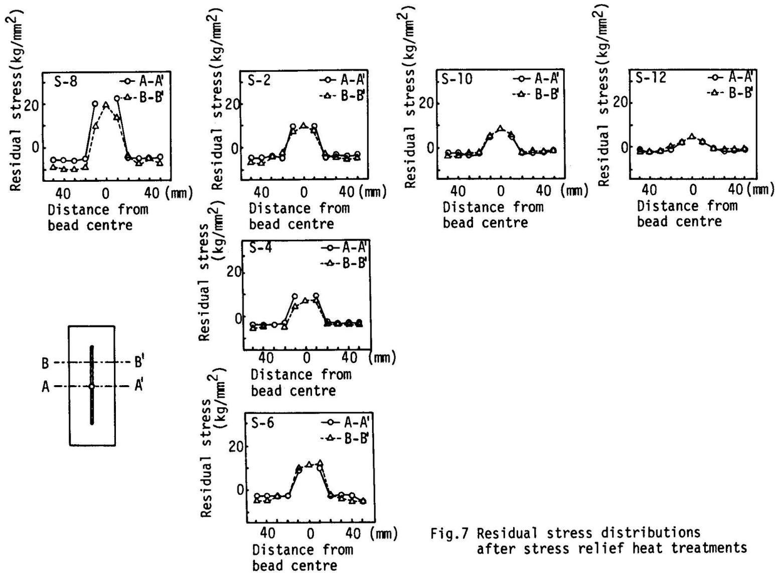
Fig.7 Residual stress distributions after stress relief heat treatments
