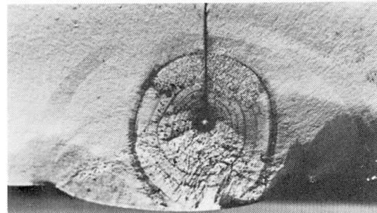
Fig. 10 Fracture Surface of Longitudinal Weld Joint
