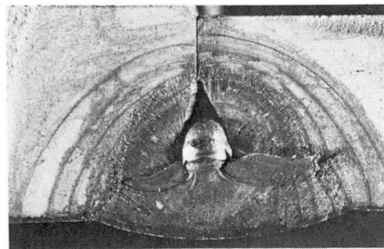
Fig. 13 Fracture Surface of Truss Lower Chord
