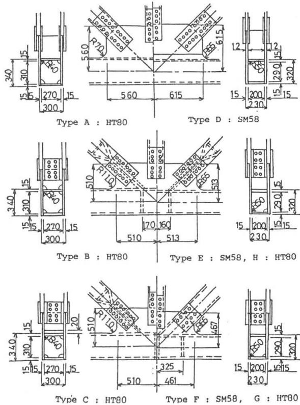
Fig. 5 Truss Panel Point Structures
