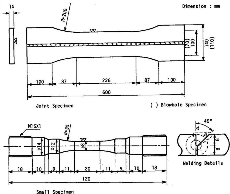
Fig. 1 Configurations and Dimensions of Specimens
