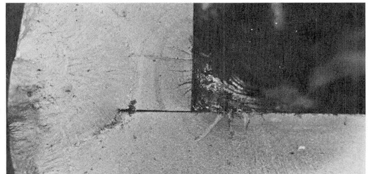
Fig. 8 Fracture Surface of Box Section Specimen
