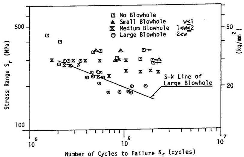
Fig. 3 Fatigue Tests Results (Influence of Blowhole)
