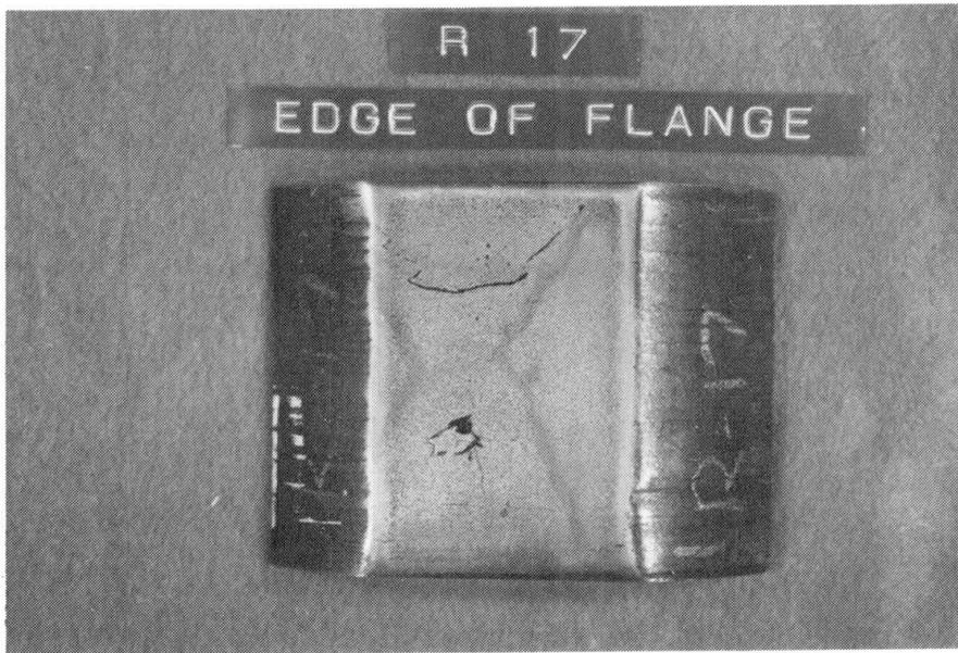
Fig. 3 Edge of Core Showing Two Defects
