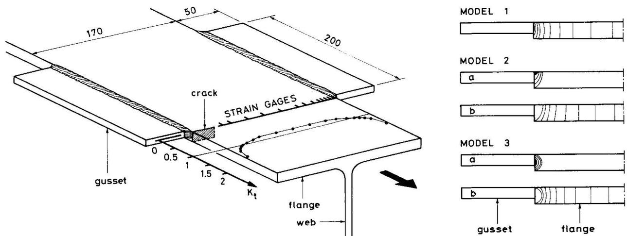
*Figure 4 : Stress concentration measurement and models of fatigue cracks emanating from the weld toe at the end of gusset plates welded to the flange tip.*
