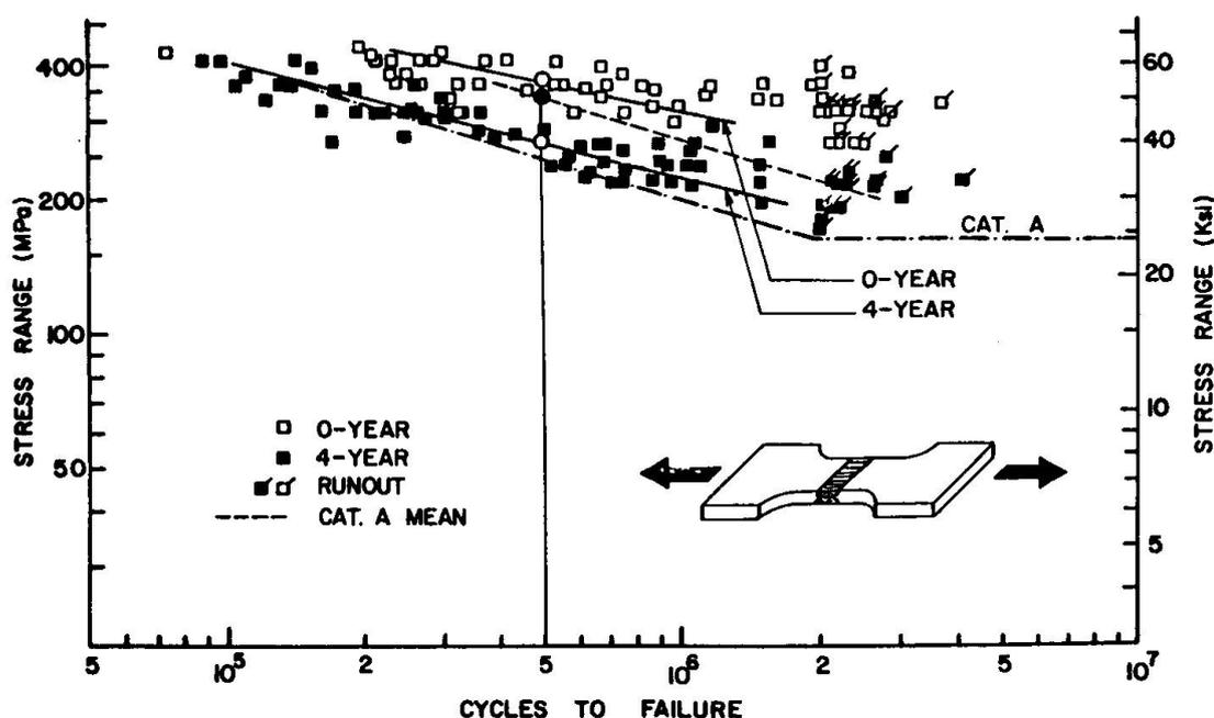
Fig. 1 Fatigue Strength of 4-Year Weathered Butt-Welded Ground Flush Specimens Fabricated from SMA steel [9].
