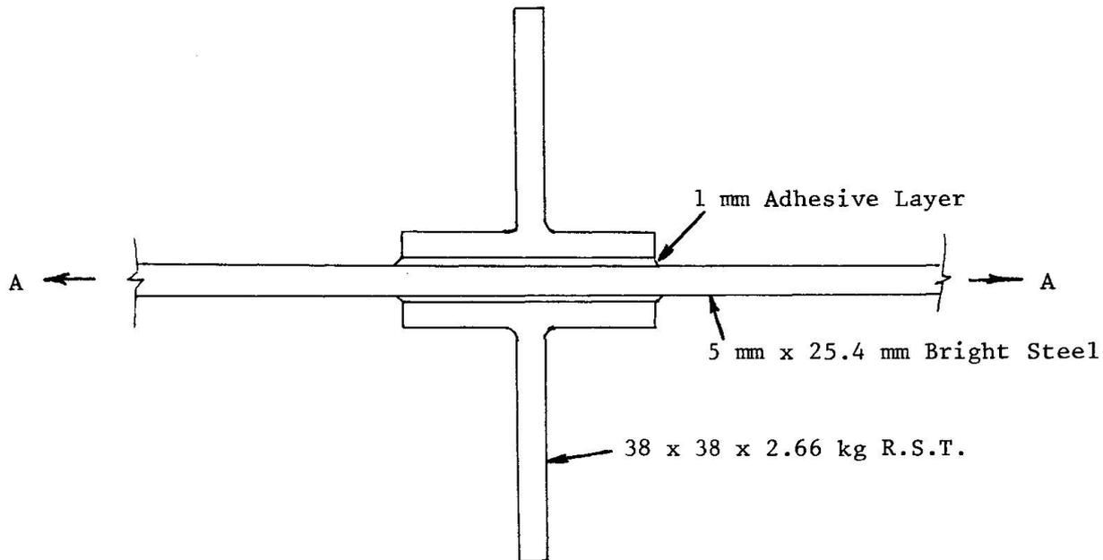
Fig 4. Test Specimen, Adhesive Bonded Unstressed T
