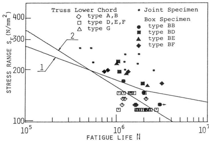
Fig. 9 Results of Fatigue Tests on Longitudinal Welds
