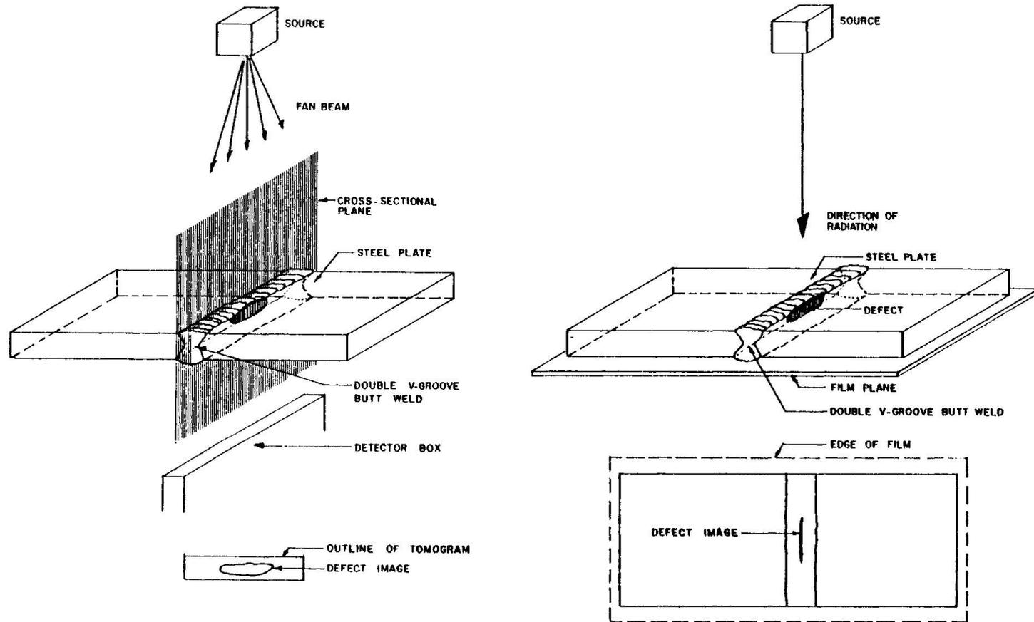
Fig. 1 Defect Imaging with CT and RT
