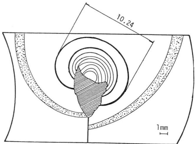
Fig. 5 Results of Beach Mark Tests (Blowhole Specimens)
