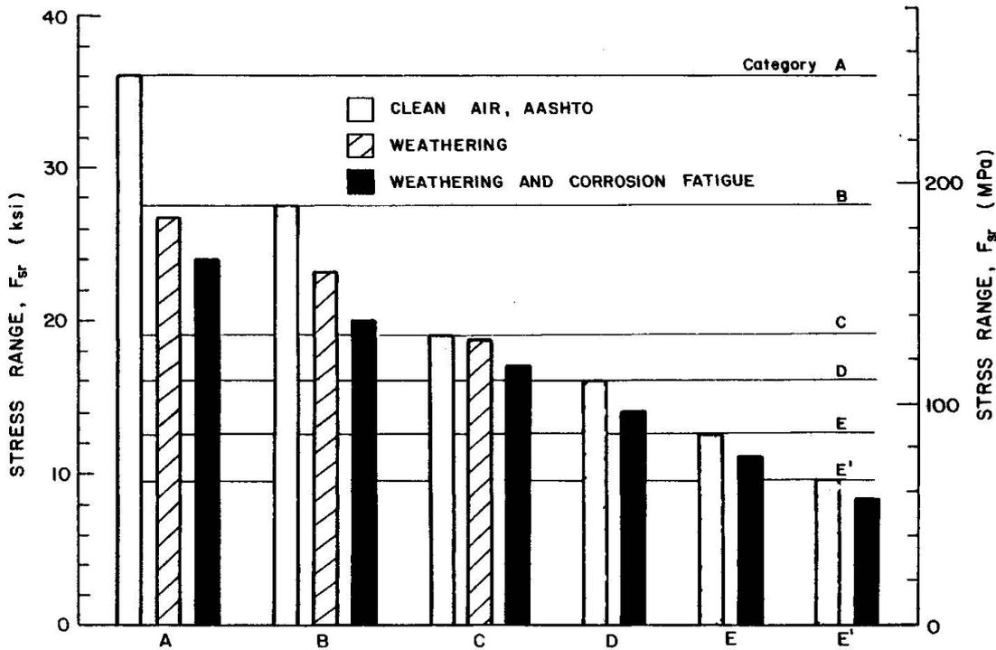
Fig. 4 Comparison of Allowable Stress Ranges for Redundant Load-Path Structures at 500,000 Cycles: (1) Current AASHTO, in Clean Air; (2) after Weathering; and (3) after Weathering and Corrosion Fatigue.
