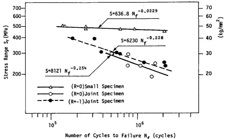
Fig. 2 Fatigue Test Results (Influence of Residual Stress)
