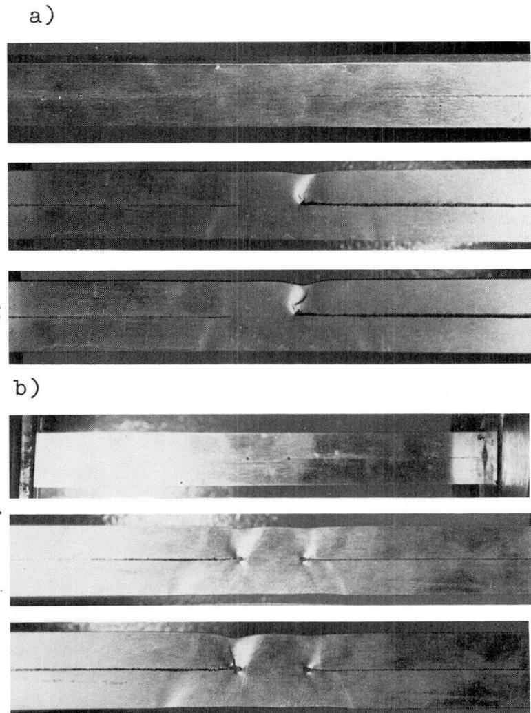
fig. 7. Static tension fracture
