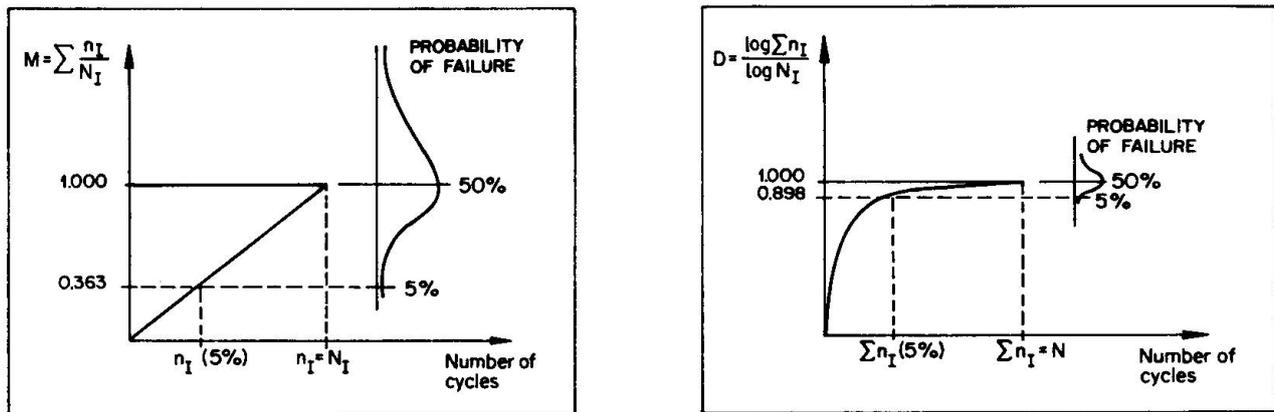
Fig.8 Interpretation of the correspondence between  $n(5\%)$  using  $M$  and  $D$  for one test of [2]
