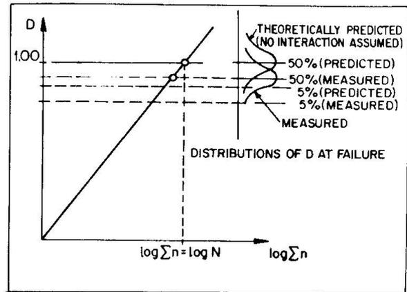
Fig. 10 Diagrammatic representation of the shift of the distribution of  $D$  for stochastic loading due to the interaction between the load levels
