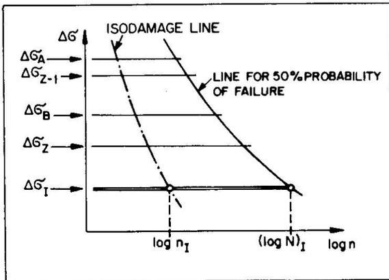
Fig. 6 Representation of isodamage lines (log. scale)
