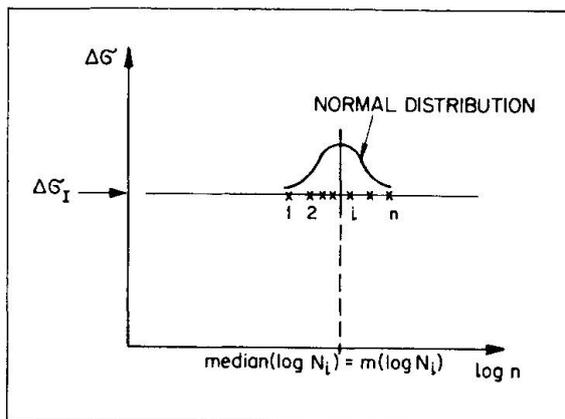
Table 1 Conversion of the number of cycles for a multi-step test at each level (normal scale)
