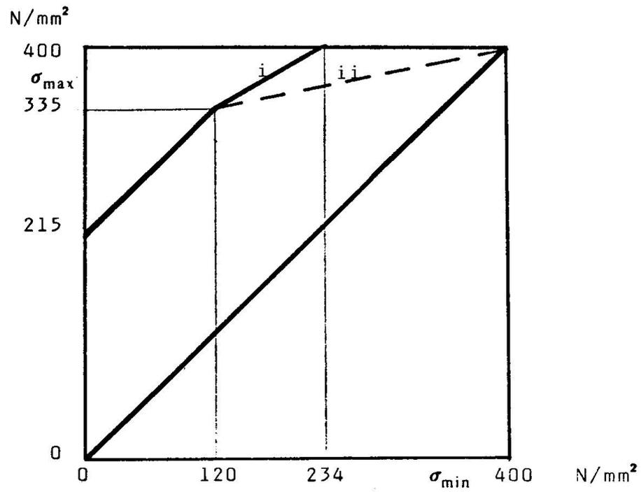
Fig. 5 Siplified modified Goodman diagram with two alternati-
