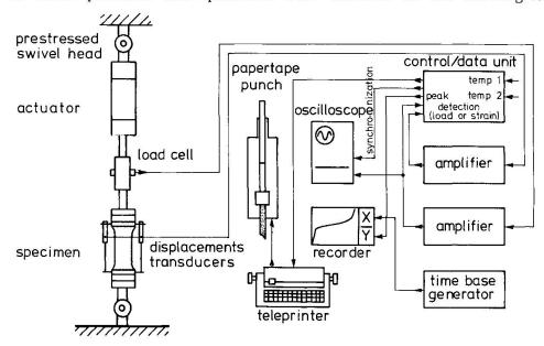
Fig. 1 Loading and controlling system (schematic)
