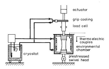
Fig. 2 Temperature control equipment
