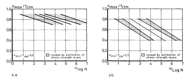
Fig. 4 Scatter in the S-N diagrams for tension (a) and tension-compression (b), as partly caused by variations of the stress-strength levels
