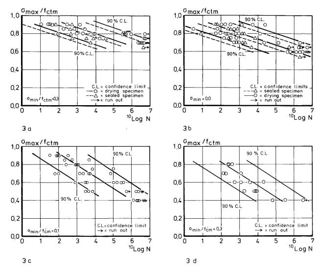
Fig. 3 S-N diagrams for dynamic tensile tests (a, b) and for tension-compression (c, d)
