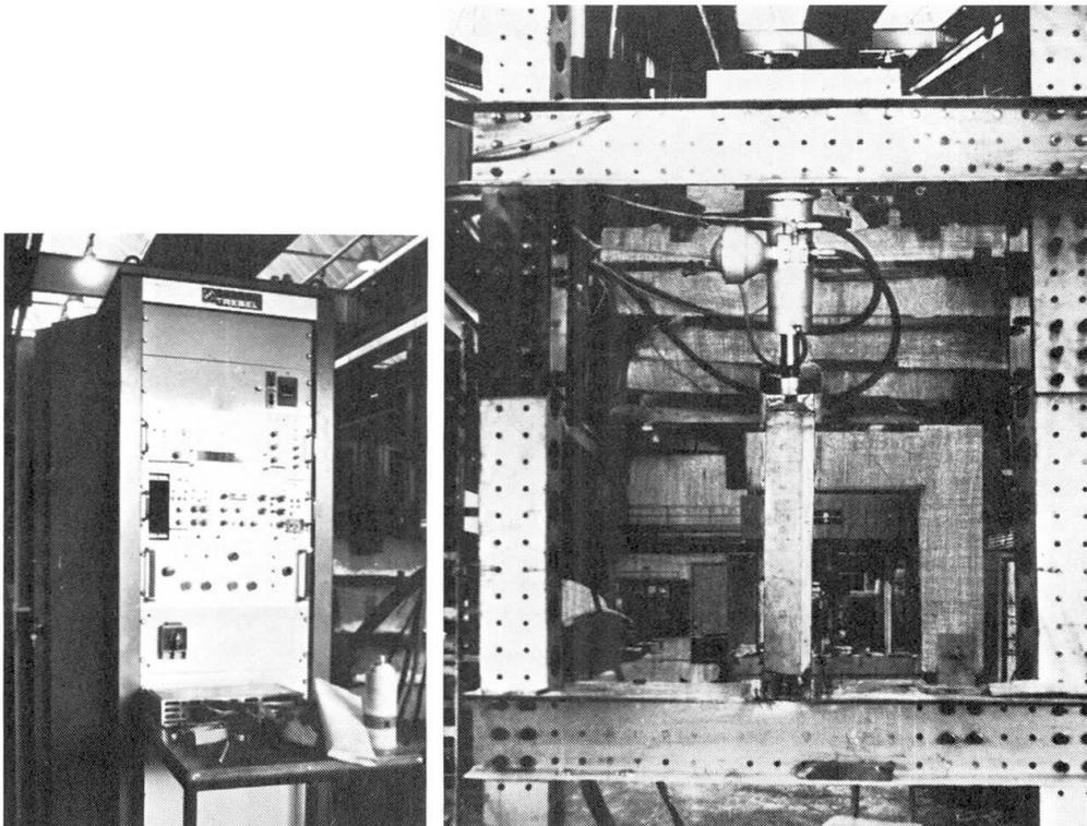
Fig. 7. Fatigue test of a concrete embedded splice
