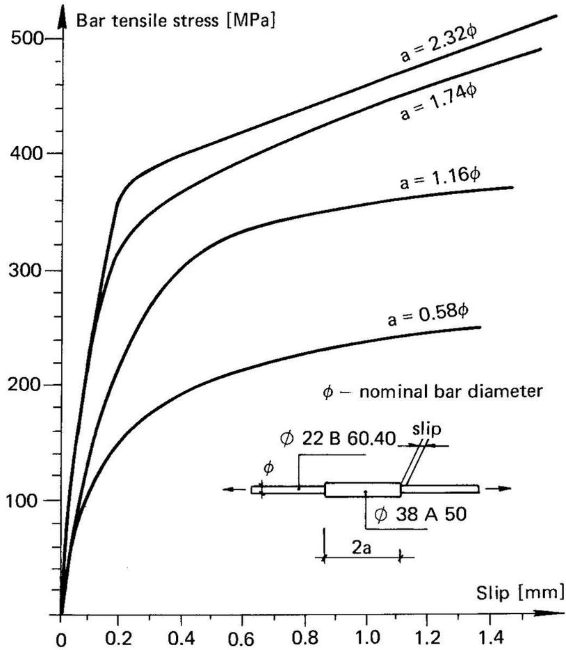
Fig. 2. Bar stress – slip relationship (single load)
