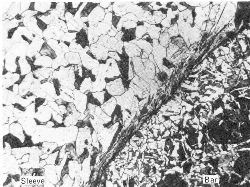
Fig. 6. Microscopy of sleeve-bar interface after fatigue test
