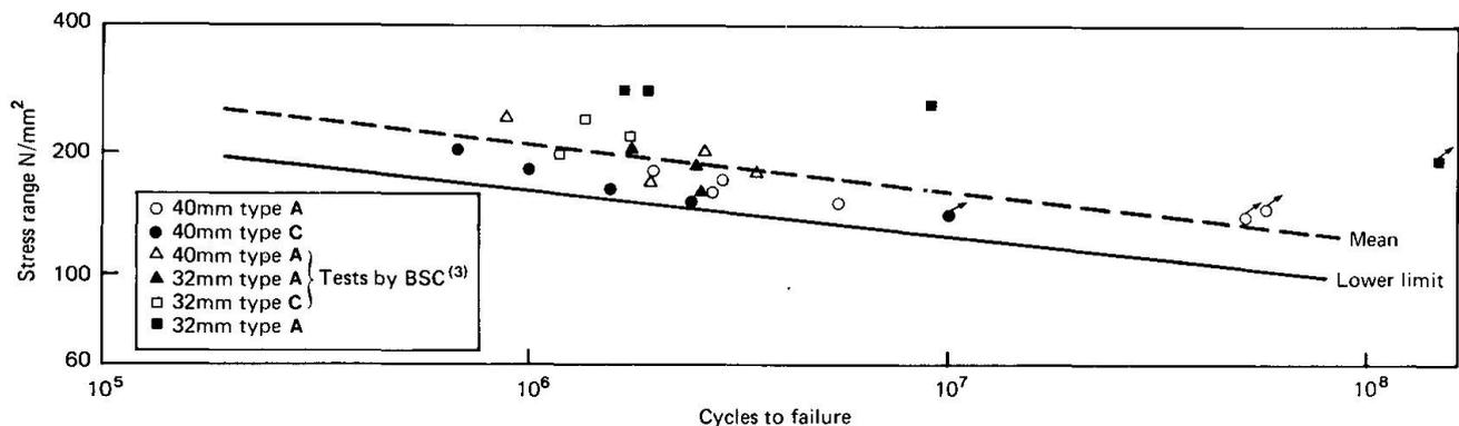
Fig.3 Performance of 32 and 40mm bars tested axially
