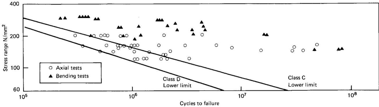
Fig.6 Performance of butt-welded bars
