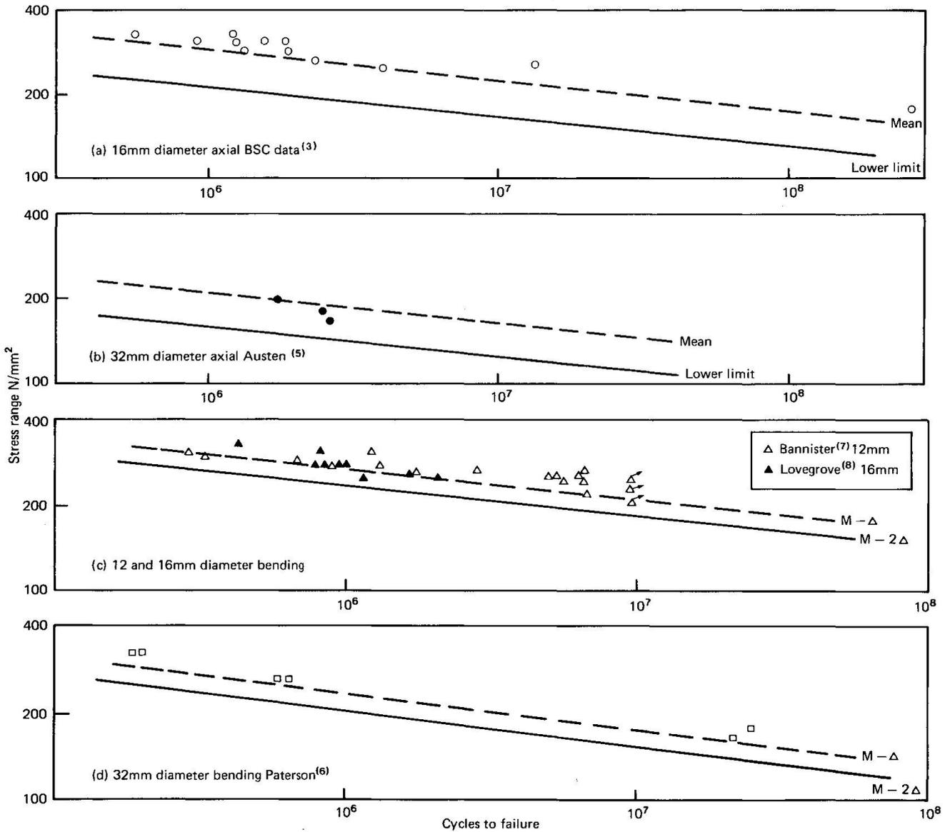
Fig.7 Comparison of performance curves with data from other laboratories : tests on type A bars
