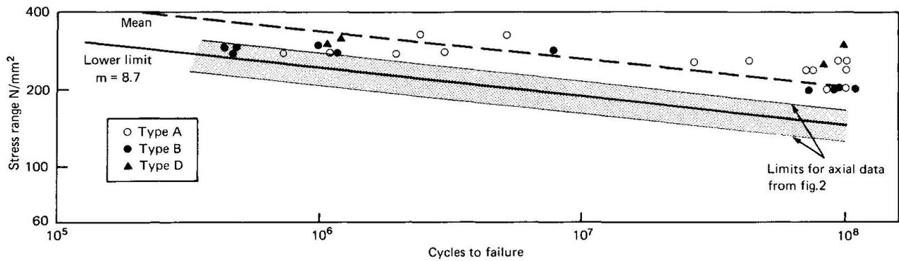
Fig.5 Performance of 16mm bars tested in bending
