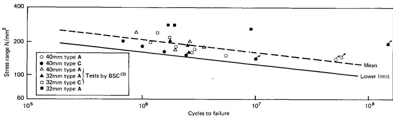
**Fig.3 Performance of 32 and 40mm bars tested axially**
