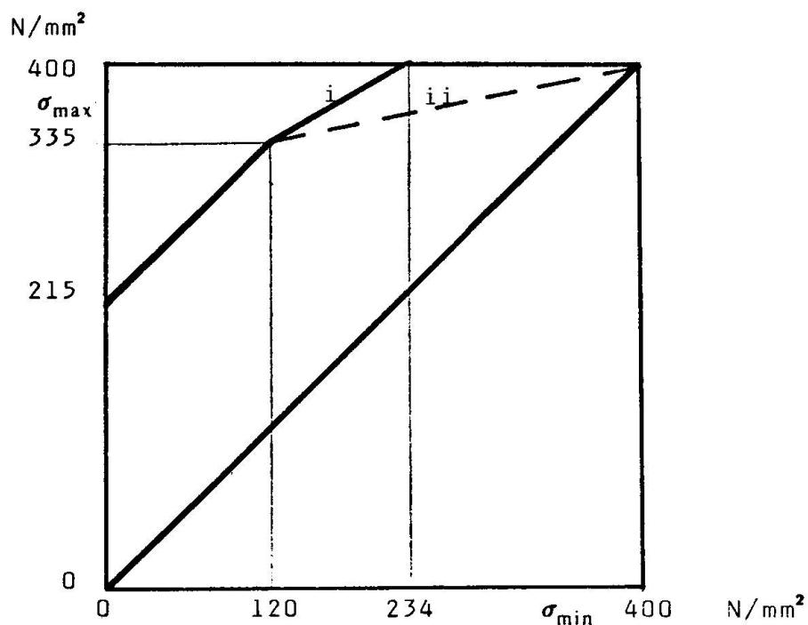
Fig. 5 Simplified modified Goodman diagram with two alternatives i and ii.
