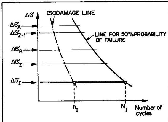
Fig. 3 Representation of isodamage lines (normal scale)
