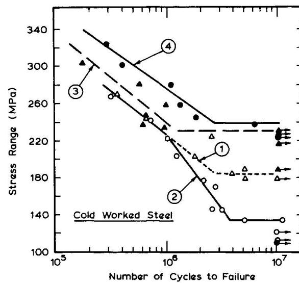
Fig. 3 S-N curves for beams
