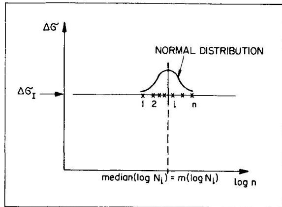
central values we carry out one-step tests on  $n$  specimens with a stress range  $\Delta\sigma_I$  as in section 2 (Fig. 5). The general expression for the new index D for test i at failure is given by
