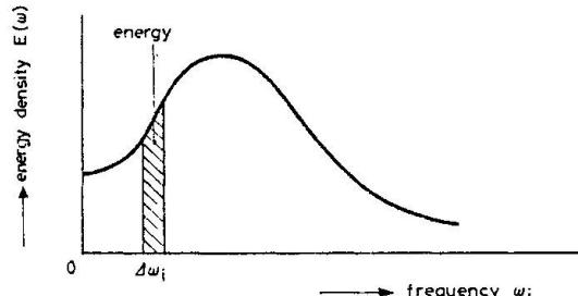
Fig. 5 Energy spectral density function
