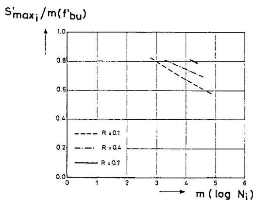
Fig. 9 Results of the Wöhler tests at 6 Hz.
