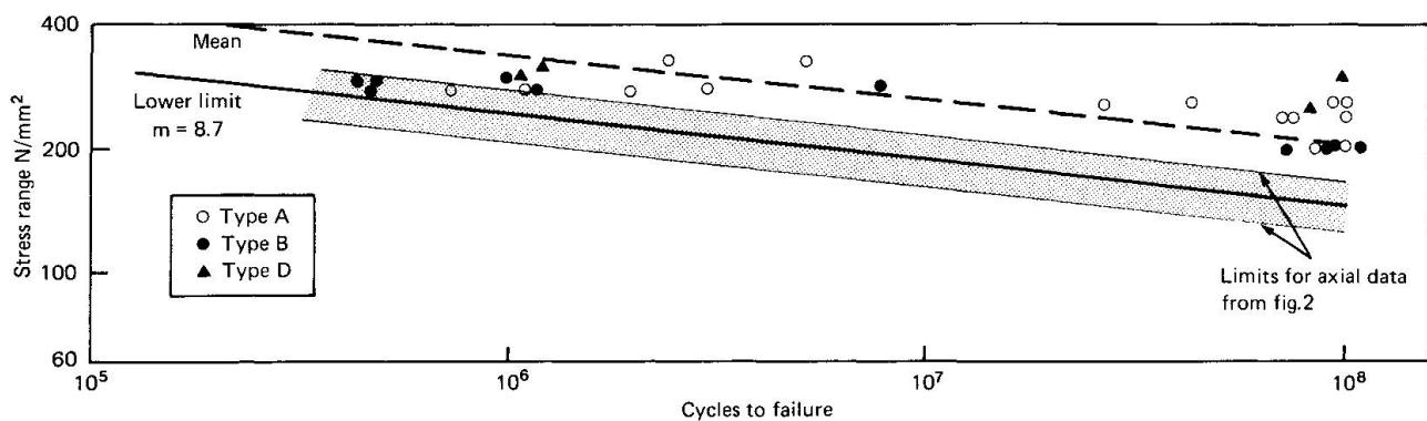
Fig.5 Performance of 16mm bars tested in bending
