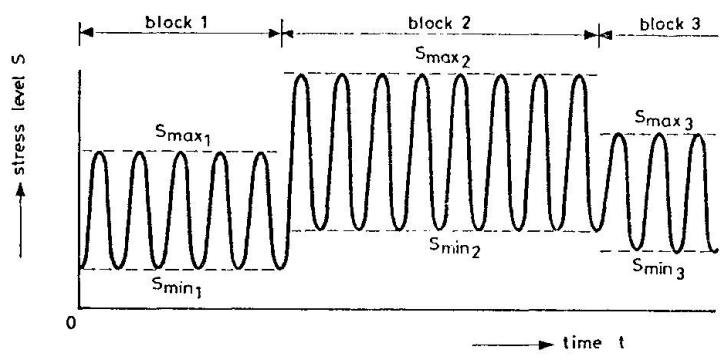
Fig. 2 Program loading test
