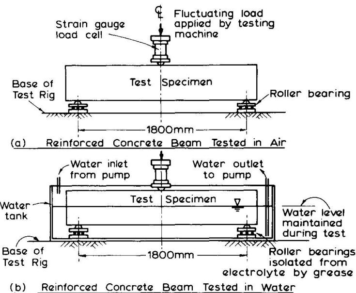
Fig. 2 Test layout of fatigue specimens
