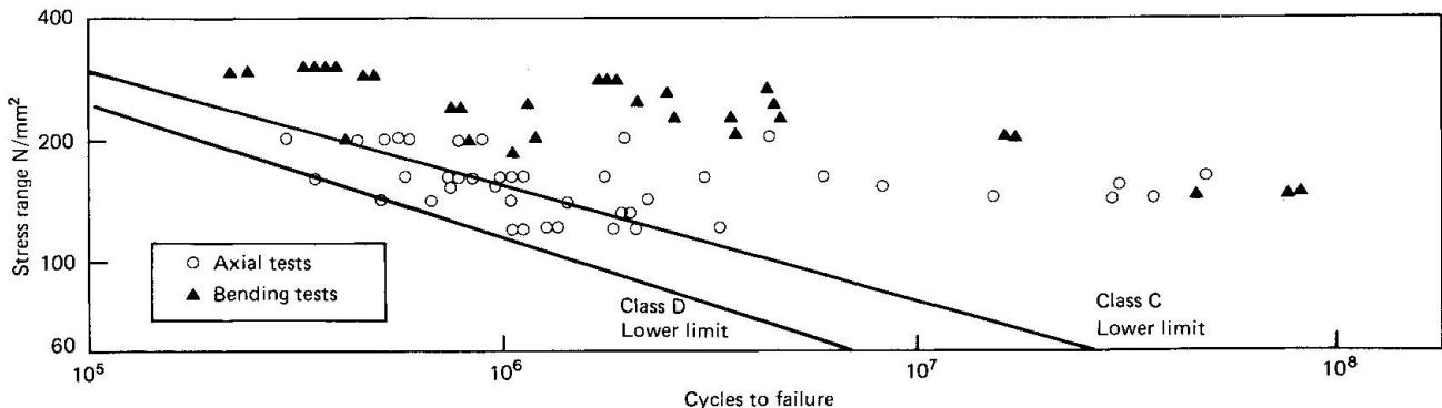
Fig.6 Performance of butt-welded bars
