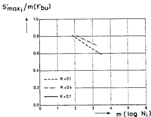
Fig. 11 Results of the Wöhler tests at 0,06 Hz
