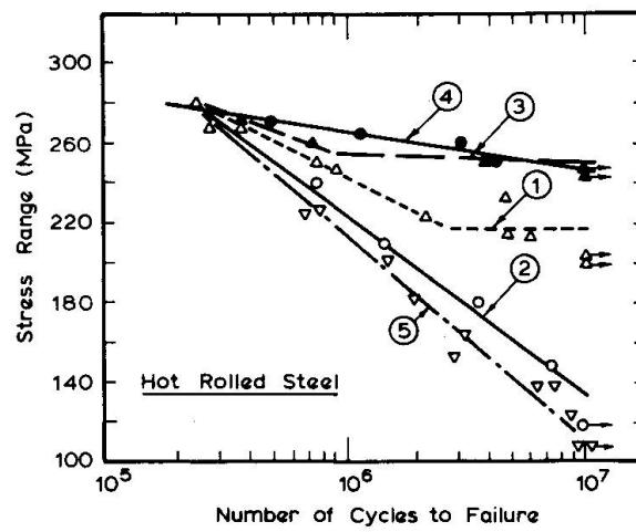
Fig. 4 S-N curves for beams
