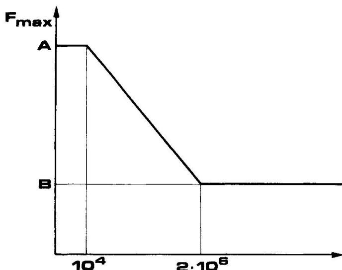
Fig. 3 Simplified effective life of the construction
