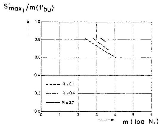
Fig. 10 Results of the Wöhler tests at 0,6 Hz.
