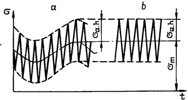
Fig.4. Loadings at pure bending compared in the work [16].
