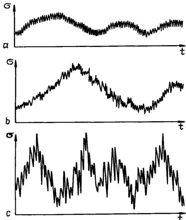
Fig.2. Change of stresses determined by oscillography: a) main beam of a bridge span  $l=23\text{m}$ ; b) in a brace of a bridge lattice girder  $l=77\text{m}$ ; when a train is passing at  $83\text{ km/h}$  speed; c) in the mast ropes.
