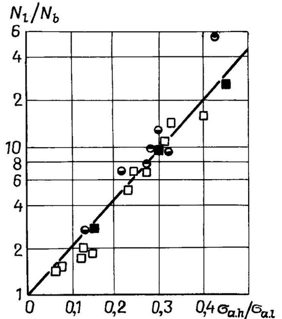
Fig.5. The generalization of testing results at two-frequency loading: □ - D16AT alloy, tension [9], ■ - D16T alloy, tension [6], ● - OX12H steel, bending [4], ● - 45 steel, bending [4].
