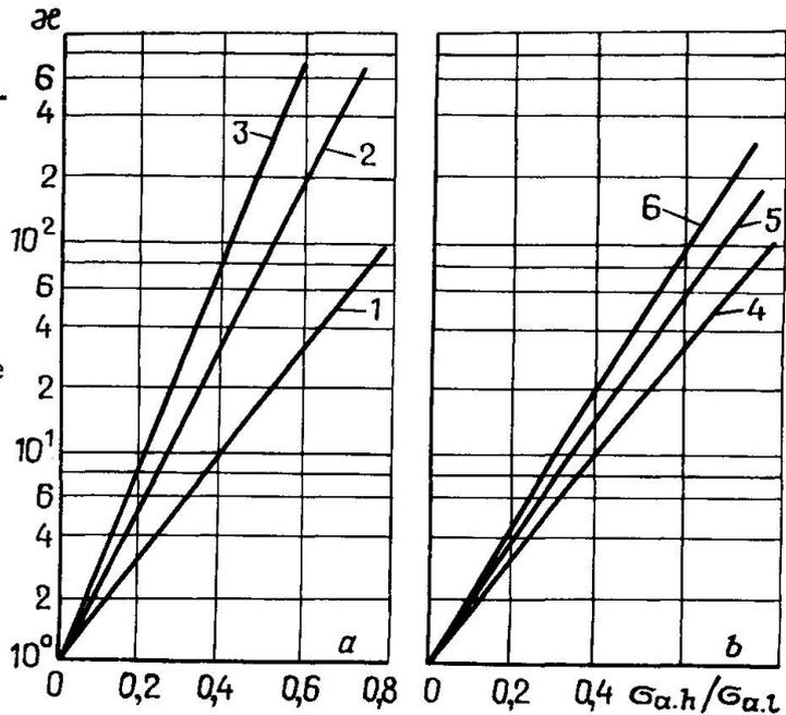
Fig.8. Relationship between  $\alpha$  and frequency ratio(a) and steel type(b): 1-  $f_h/f_l = 10^2$ ; 2-  $f_h/f_l = 10^3$ ; 3-  $f_h/f_l = 5 \cdot 10^3$ ; 4-low-carbon steel; 5-chrome-nickel steel; 6-high-strength steel.
