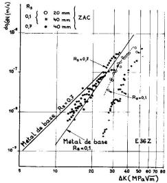
Figure 3 Evolution de da/dN = f ( $\Delta K$ ) Figure 4 Evolution de da/dN = f ( $\Delta K$ ) Acier E24
