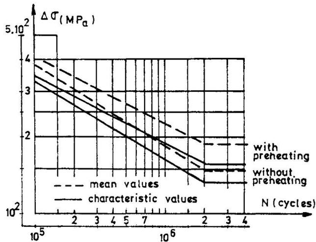
Figure 7. Fatigue tests results with and without preheating.
