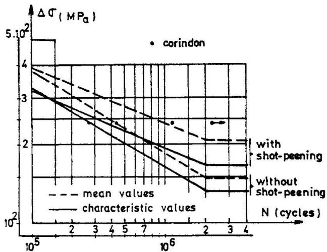
Figure 6. Fatigue tests results with and without shot-peening.
