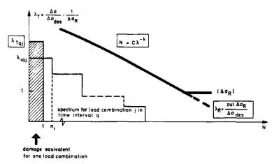
Fig. 3 Computing  $\lambda_{Tqj} = \left[\sum n_i \lambda_{iqj}^k\right]^{1/k}$  the fatigue damage equivalent stress amplitude (depending on material, notch and component / system characteristics -  $\Delta \sigma_R$  - and relative to the specification load spectrum -  $S_3$ :  $\Delta \sigma_{des}$  - )
