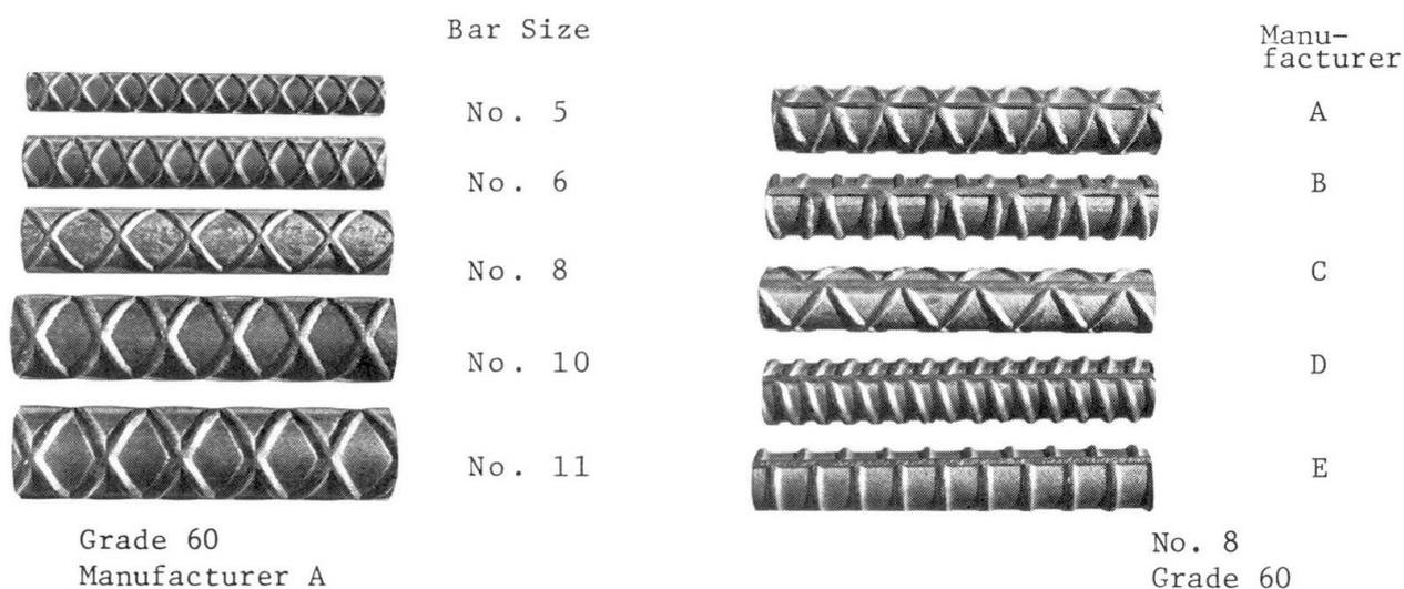
Fig. 1 Reinforcing Bars Used in Test Program
