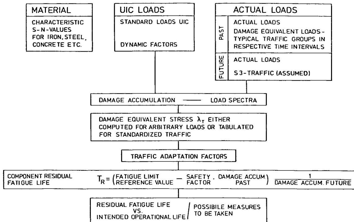
Fig. 1: Computation scheme for residual fatigue life
