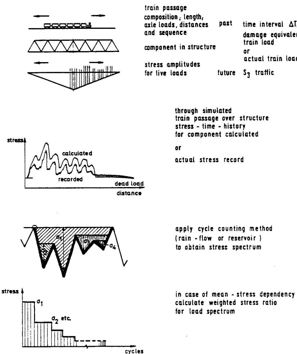
Fig. 2: Computation of load spectrum for structural component
