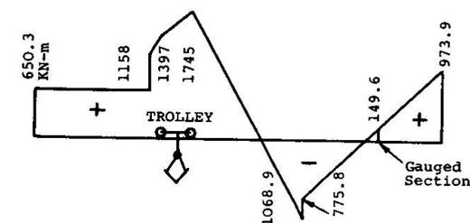
Fig. 7 Boom B.M. for Trolley in Working Position
