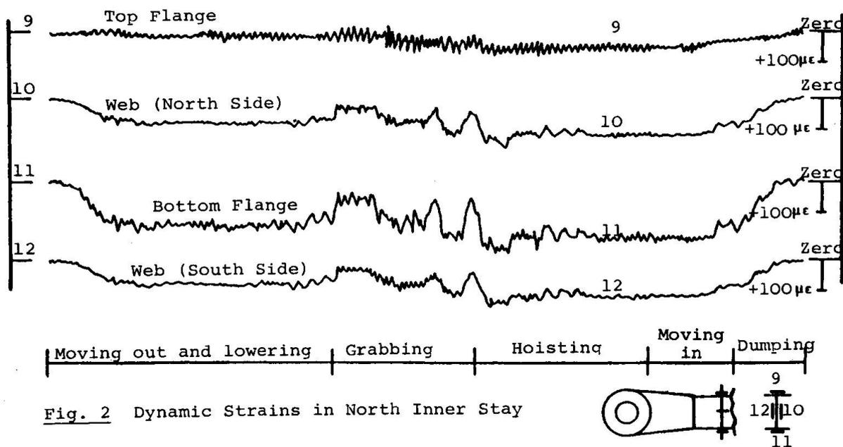
Fig. 2 Dynamic Strains in North Inner Stay
