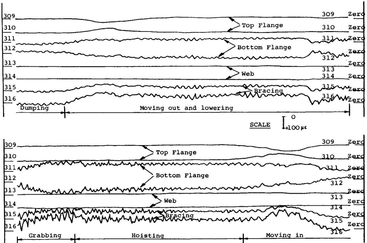
Fig. 5 Dynamic Strains in Repaired Joint Structure.
