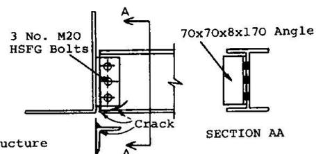
Fig. 3 Details of Original Joint Structure
