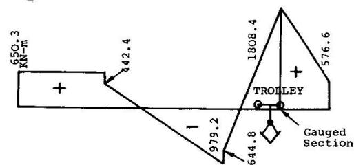
Fig. 8 Boom B.M. for Trolley passing Gauged Section
