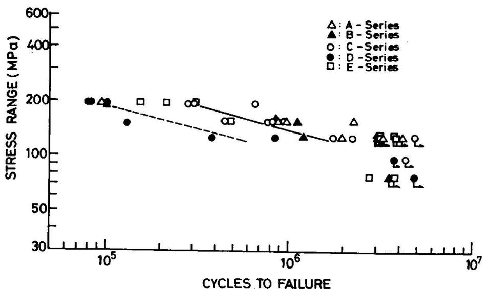
Figure 3: Fatigue test results of tensile specimens.
