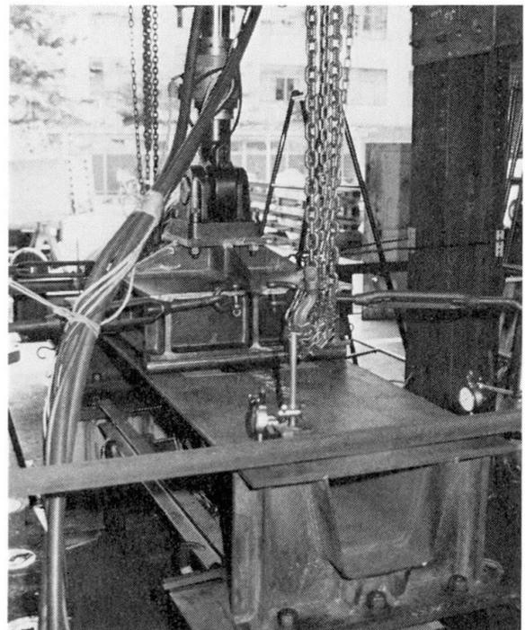
Photo 1: Test set-up for bending fatigue test.
