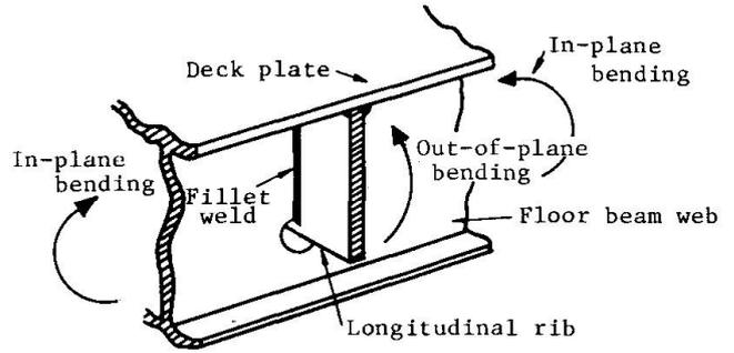
Fig. 12 Bending condition in floor beam web
