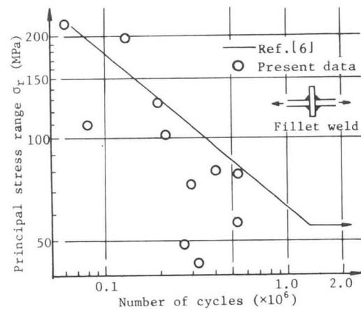
Fig. 18 S-N relations of fillet welded joint
