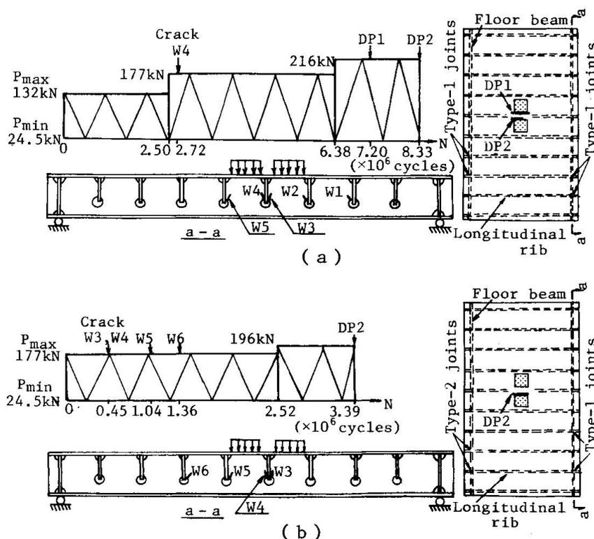
**Fig. 5** Testing records and locations of cracks
