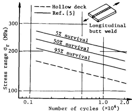
Fig. 16 S-N curves for butt welded joint
