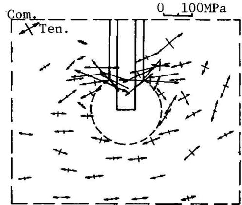
Fig. 13 Principal stresses in floor beam web
