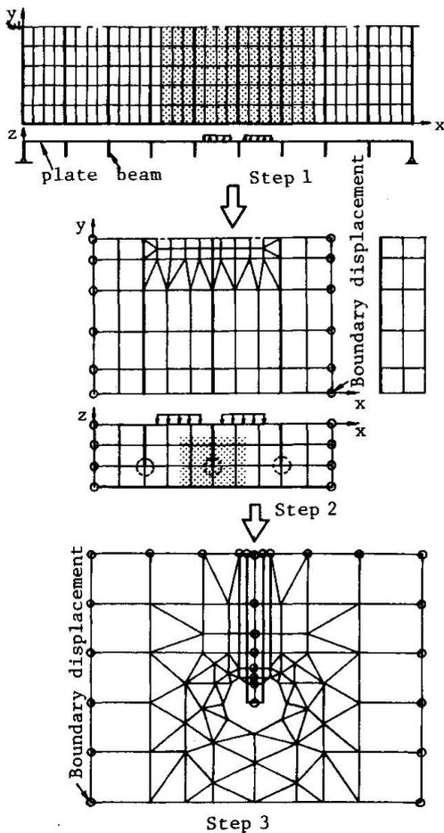
Fig. 11 Finite mesh divisions at zooming step
