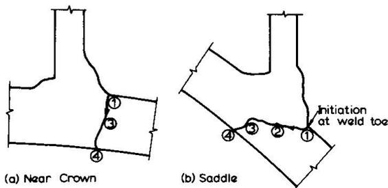
Fig. 5 Specimen 1: Through Wall Crack Paths
