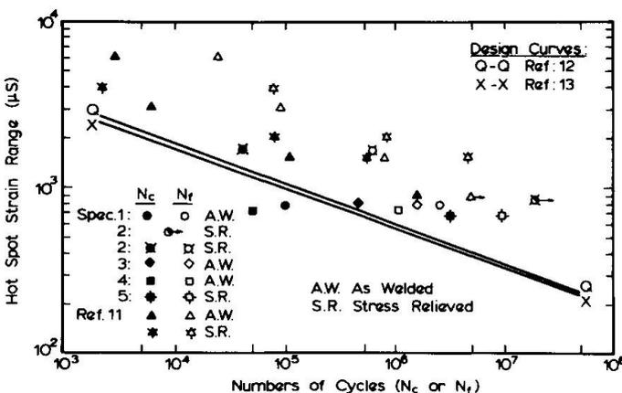
shown in Fig. 3 is the as-welded and stress relieved fatigue data of Yamaski et al. [11] who concluded that stress relieving had no influence on fatigue strength. Although statistically not significant two of their specimens tested at the same load range clearly show a superior fatigue strength for the stress relieved specimen. One further remark about the cited work is that most of the specimens were tested at higher strain ranges at which the influence of residual stresses will be reduced.
