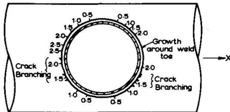
Fig. 4 Specimen 1: Crack Growth in Millions of Cycles
