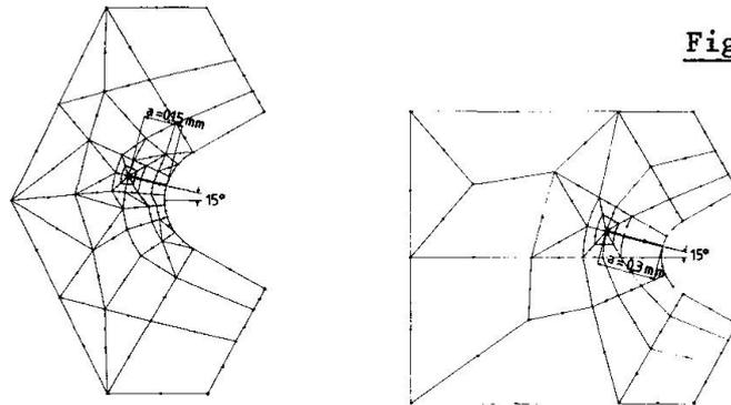
Fig. 5 Local FE models of the most stressed notch of the cracked bolt thread
