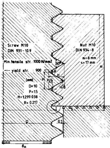
**Fig. 1** Threaded connection M10
