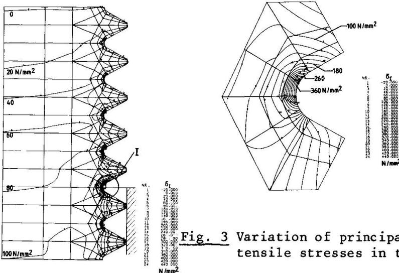
**Fig. 3** Variation of principal tensile stresses in the bolt
