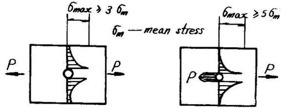
(a) Plate with a hole (b) Joint with a rivet
