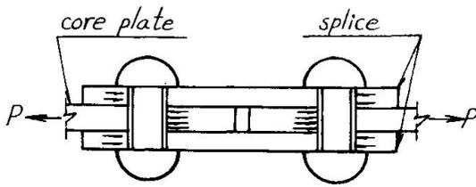
Fig. 3 Manner of force transmission of riveted joint
