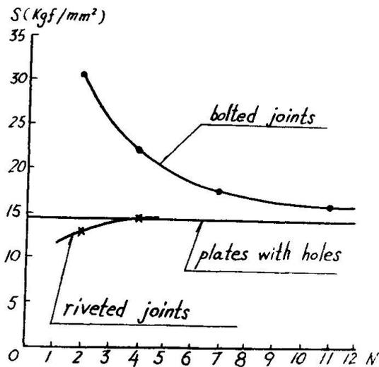
**Fig.2** Relationships between fatigue strength of joints and number of fasteners in a line (R=0, 2x10<sup>6</sup> cycles)
