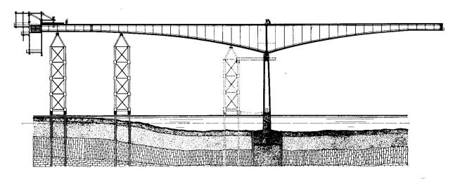
The free cantilevering may appear a daring way of construction, but it does in fact permit the bridge to grow in a simple and natural way. As the cantilever moment grows bigger, the prestressing force is increased, and properly designed one can maintain almost uniform stress from deck to soffit of the cross section, and thus in spite of a very large dead weight moment have rather small resulting deflections.
