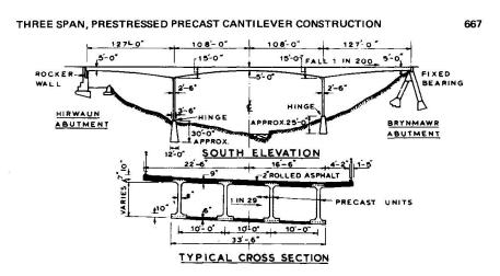
Each box section consisted of 4 No.I-sections and with the bridge spans being symmetrical it had been assumed there would 16 No.
