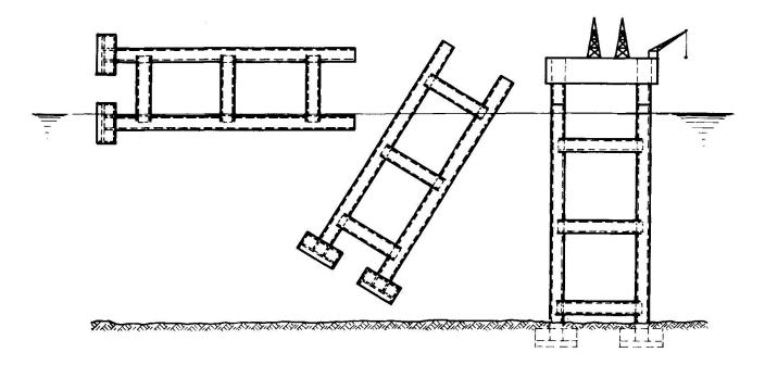
The tower may rock about a bit in the waves; but it is possible to live and work comfortably inside the structure from the moment of touch down, and it would not appear too difficult to develope a firm foundation somewhere between huge piles or nothing, which would make sense in ordinary geotechnical terms. This may require some new and specialist equipment, but surely nothing as outrageous as hammers weighing hundreds of tons or cranes with capacities of thousands of tons.
