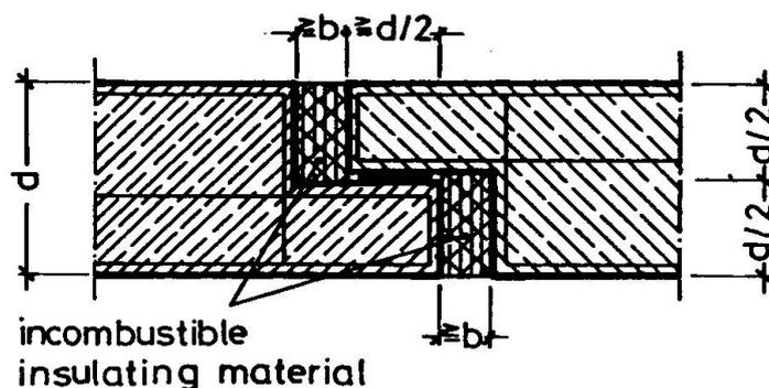
Fig. 12 Proposal for the Design of an Expansion Joint with High Fire Resistance Properties
