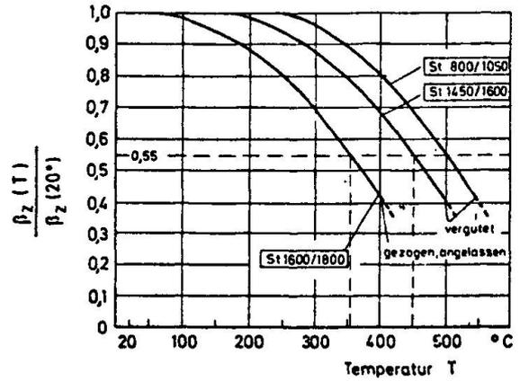
Fig. 3 Tension Strength of Pre-stressing Steel vs. Temperature
