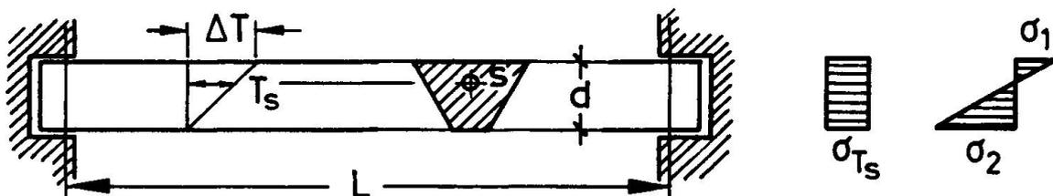
Equal temperature distribution over the whole length  $L$ , linear temperature gradient  $\Delta T$ :
