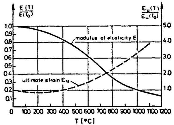
Fig. 5 Modulus of Elasticity and Ultimate Strain of Reinforcing Steel vs. Temperature
