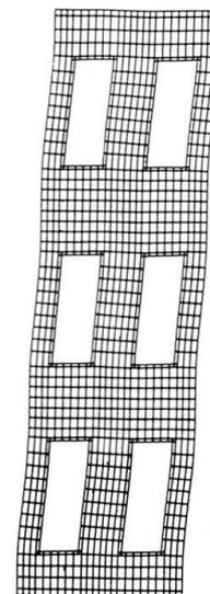
FIGURE 12 - DEFORMED SHAPE OF EXTERIOR WALL
