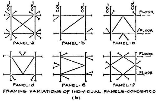
Generalized layouts of normal braced frames with (a) showing general layout where each individual panel may have various configurations as shown in (b).
