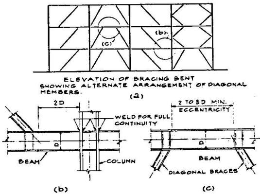
"Braced frame" bracing arrangements using eccentric connections to absorb energy. (a) Elevation of bracing bent showing alternate arrangement of diagonal members. (b), (c) Enlargements of areas shown in (a).
