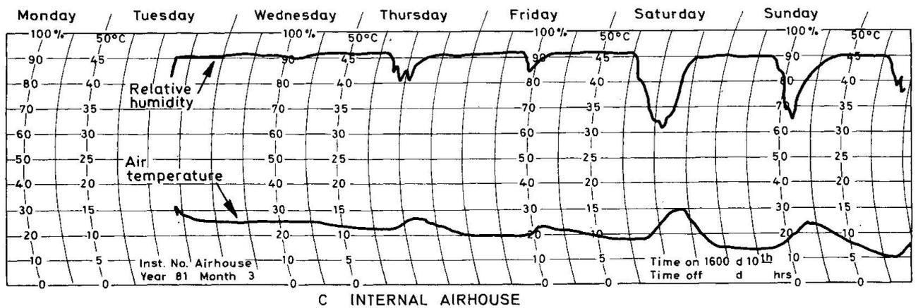
Figure 7. Dry bulb temperatures and relative humidities
