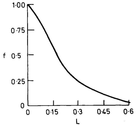
Figure 8 (a) Relationship between conductance–capacity index, decrement factor and time lag for different materials
