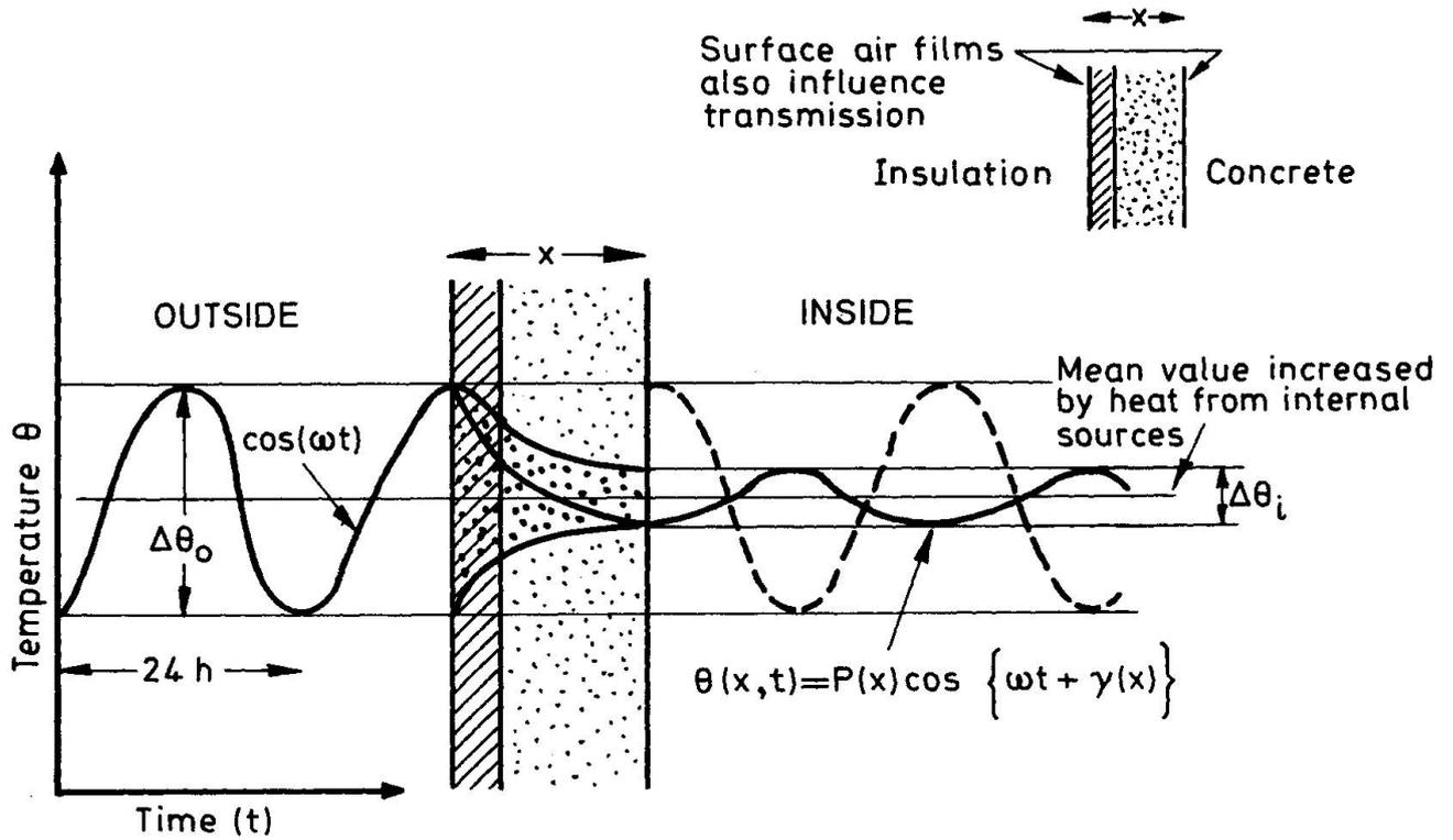
$P(x), \gamma(x)$  are thermal properties of the construction
