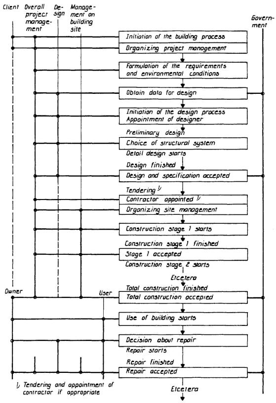
FIG.1. Stages of the building process showing interactions
