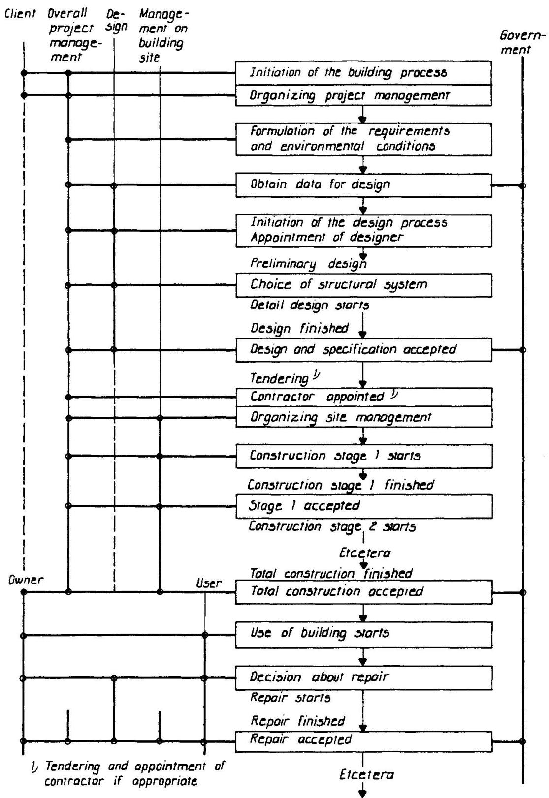
FIG 1 Stages of the building process showing interactions
