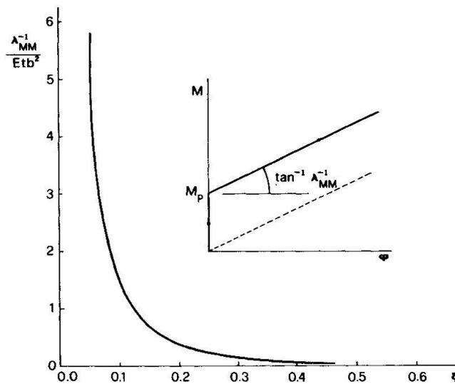
Fig. 5 Hardening coefficient against relative crack depth.
