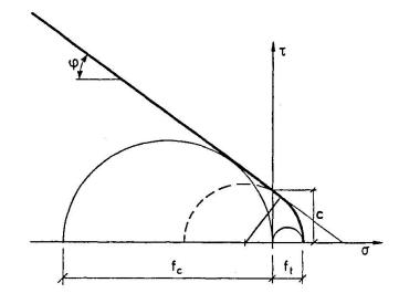
Fig. 1 Modified Coulomb failure criterion
