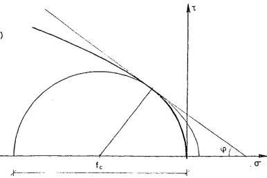
Fig. 8 Parabolic failure envelope with zero tension cut-off.
