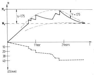
$\frac{\text{Fig. 7}}{\text{actions}} \text{ Time depending restraint actions due to settlements}$
