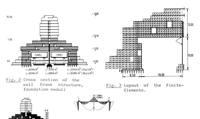
Fig. 5 Variation of the support-moment due to elastic supports.
