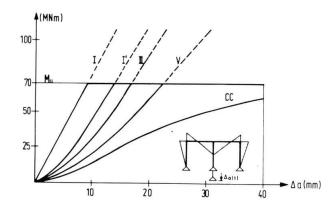
Fig. 6 Structure responses to differential settlements
