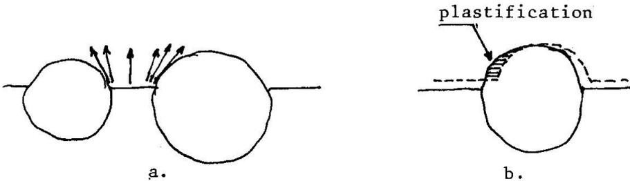
So there is a certain range of freedom as far as the crack opening direction is concerned. Only a limited number of particles will be found providing planes of resistance, perfectly perpendicular to the crack plane (Fig. b). In such a case deformation of the relatively soft matrix will occur, so that shear displacement is not prevented. So from a physical point of view we can expect a shear displacement component to occur already at zero-crack width. This was also confirmed by our tests.
