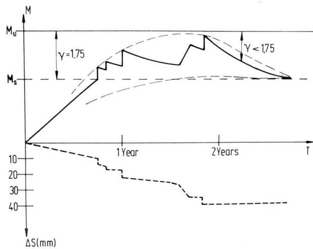
Fig. 7 Time depending restraint actions due to settlements
