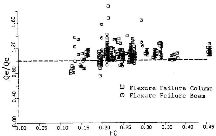
Fig.11 Flexure Failure Specimens Subject to Anti-symmetrical Bending
