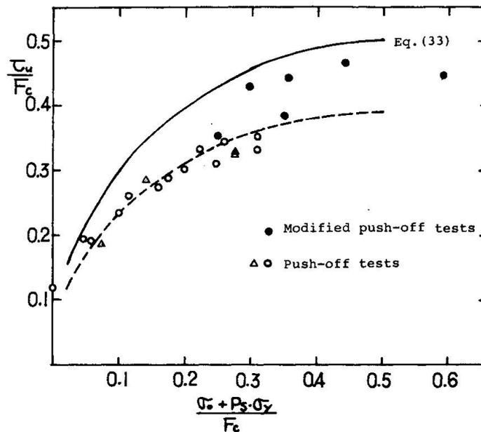
Fig.15 Comparison Between Test Results and Calculated Values
