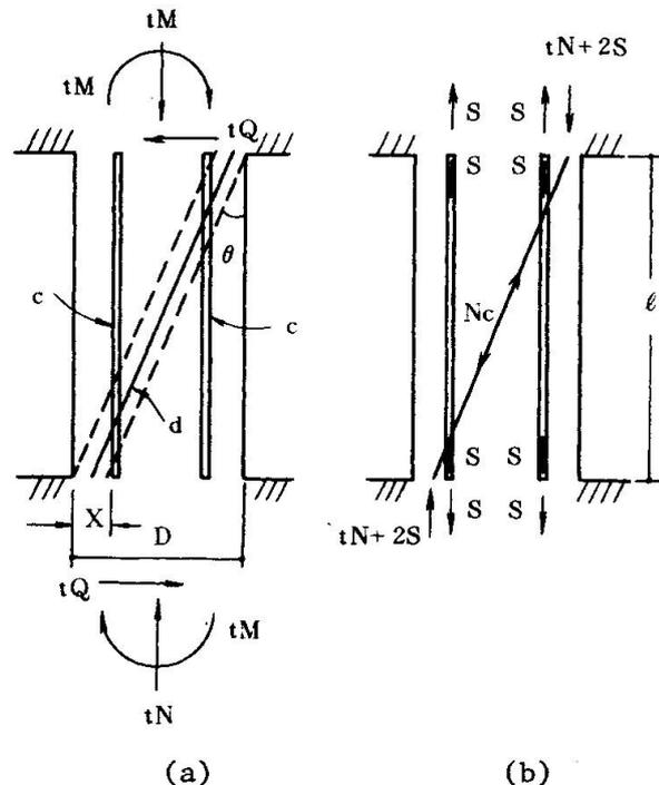
Fig.3 Compression Field Model Subject to Anti-symmetrical Bending
